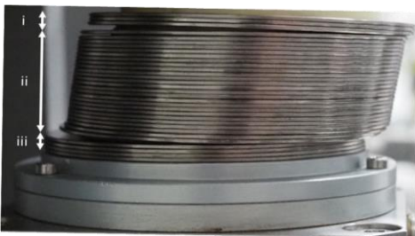
Figure 1. A result at the end of an OC DSS test with slippage.
