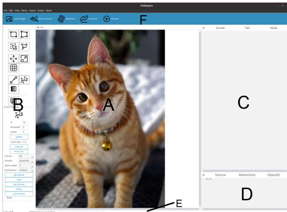
Figure 28. FoldingGen interface layout. The interface consists of (A) Canvas(with input image imported), (B) Toolbox Panel, (C) Jump Path Tree, (D) Motion Zone Panel, (E) Status Bar, and (F) Workflow Panel.
