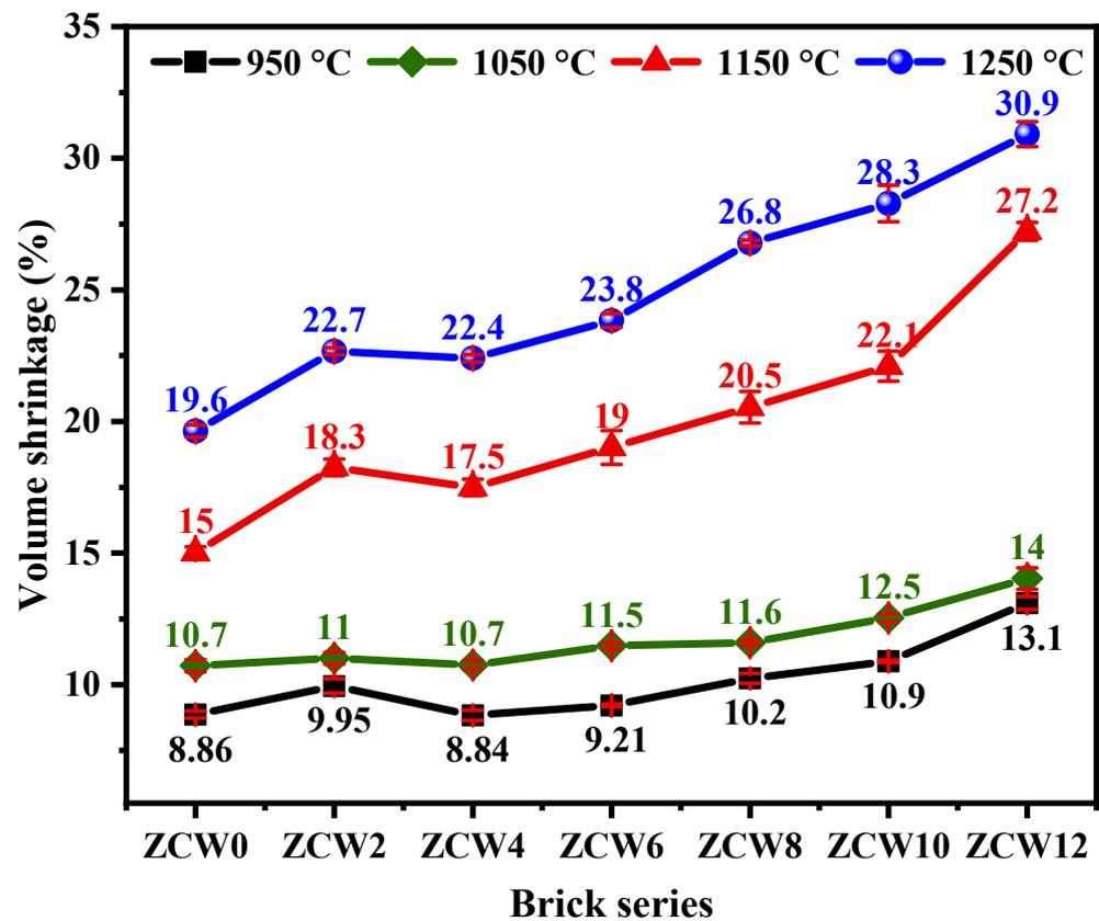
Figure 14. Volume shrinkage of the developed bricks under different sintering temperatures.
