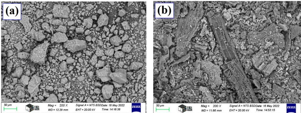
Figure 5. SEM photos of (a) zeolite tuff and (b) cigarette waste.
