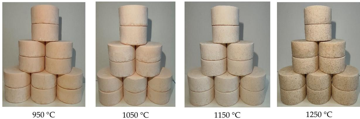
**Figure 9.** Produced bricks at different temperatures.
