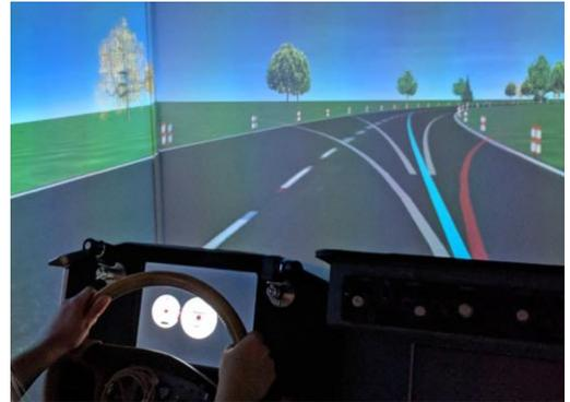
Fig. 2. Visual feedback design as implemented in the simulator, with future trajectory curves forming the performance envelope.
