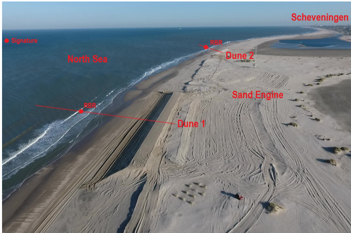
Figure 3.5: The layout of the RealDune-REFLEX field measuring site. The measurement devices are shown with their respective location and orientation to Dune 1 and Dune 2. The RBR sensors are located on the mid-transect for Dune 1 and Dune 2. The Signature ADCP (depth d \approx 14 m) and the Europlatform (depth d \approx 32 m) are located offshore. The Europlatform, tidal gauge of Hoek van Holland and the tidal gauge of Scheveningen are not depicted in this figure.
