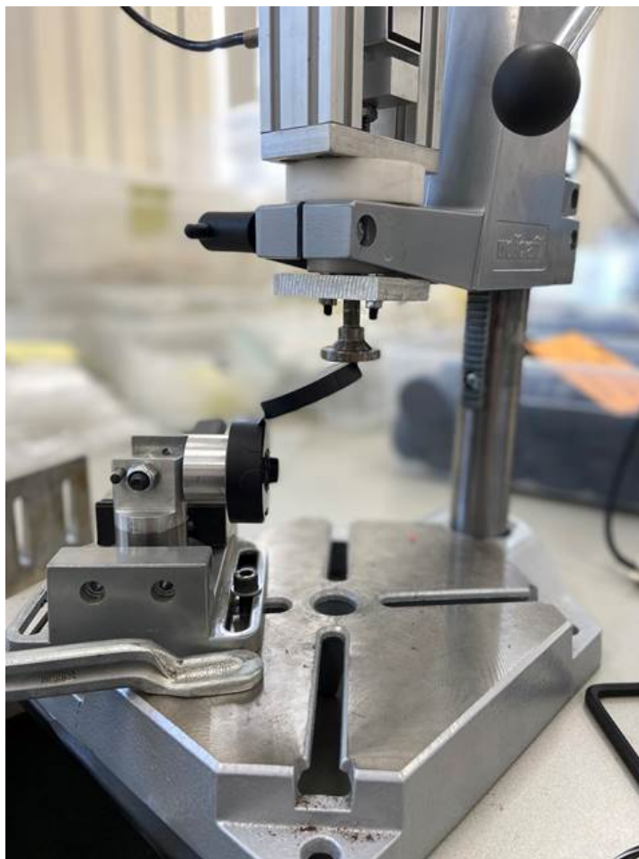
Figure 2.2: uniaxial compression test on the closure
