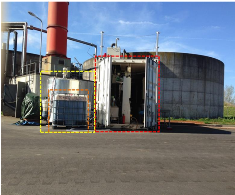
Figure 1. Impression of the pilot plant. The open container contained the selector and accumulator bioreactor (red bracket). In the front, there is an IBC sedimentation tank (orange bracket). Behind the sedimentation tank, the influent buffer vessel was located (yellow bracket). (Image by Michel Mulders.)
