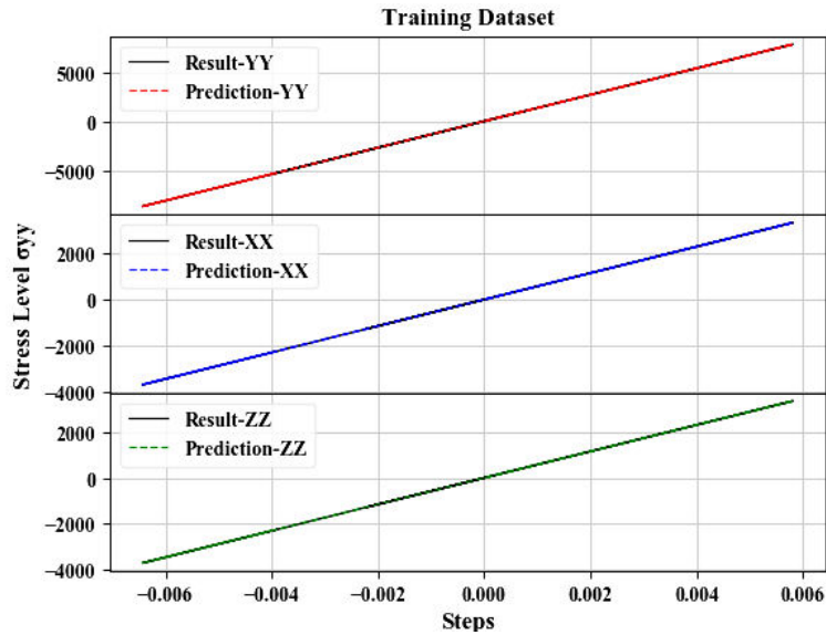
Figure 82 The results of the Neural Network with 3 directions as outputs. Stress Vs Strain
