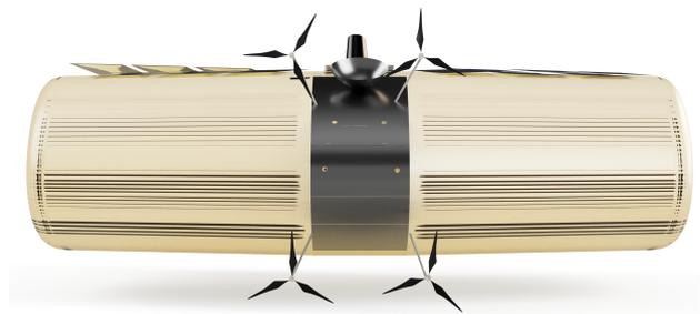
**Figure 3.11:** Propeller placement
