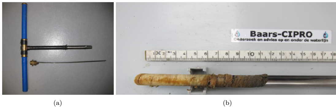
Figure 2.3: An increment borer (a) is used to take a wood sample (b) from the pile (De Gijt and Roubos, 2013), (Baars-CIPRO, 2019).
