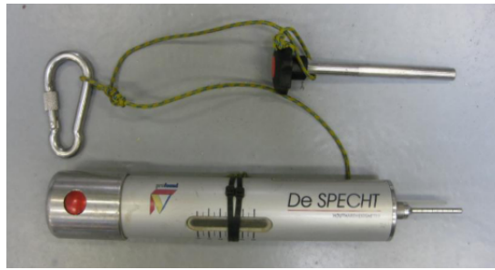
Figure 2.5: Penetration meter: Specht De Gijt and Roubos (2013).
