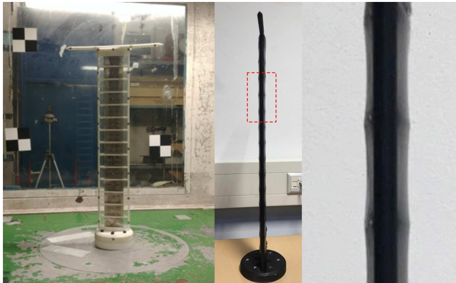
Fig. 1 Pazy Wing in wind tunnel at Technion (left) [1]. Outer surface of the Pazy Wing from TU Delft in undeflected jig-shape with close up highlighting the sagging skin (foil cover) between the ribs.
