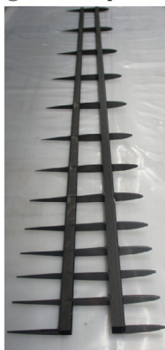
(e) Bonded skeleton consisting of spars and ribs.
