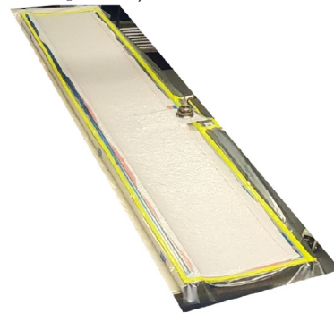
(d) Vacuum bagging of the top skin of the wing.
