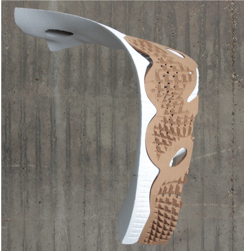
Figure 1 Hybrid of cork and expanded polystyrene, the prototype has a built-in hybrid behaviour that extends material properties of the two materials
