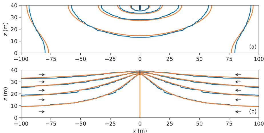
**Figure 2.** Cross-section of flow to a partially penetrating canal in an aquifer consisting of 400 layers for the stratified model with one random realization of layer properties (blue) and the homogeneous model with uniform  $k_h$  and  $k_v^*$  (orange); (a) head contours with contour interval 2 cm and (b) streamlines with contour interval  $Q/10$ .
