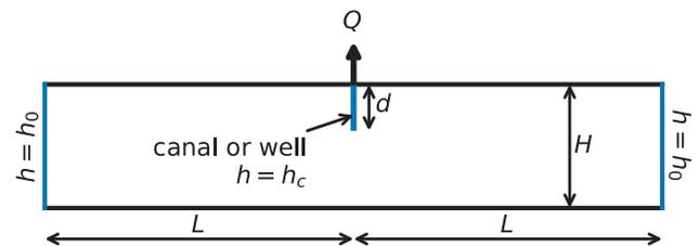
**Figure 1.** Cross-section of flow domain used for the numerical experiments (not to scale). Flow domain may represent two-dimensional flow towards a partially penetrating canal or radially symmetric flow to a partially penetrating well.
