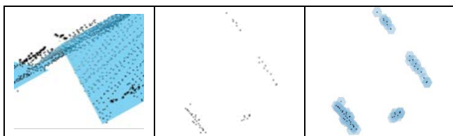
Figure 1. Obstacle detection based on geometry mismatches between the datasets (left to right: highlight of the most distant points, selection, offset)
