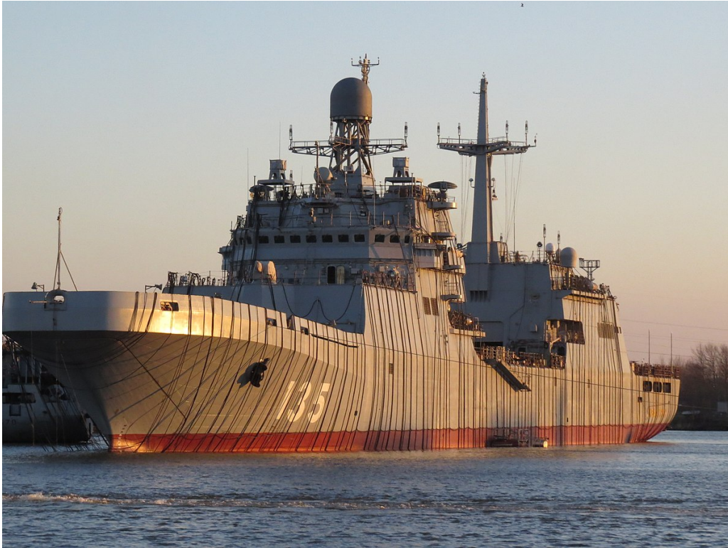
Figure 1.2: A naval vessel is being depermed at a harbour.
