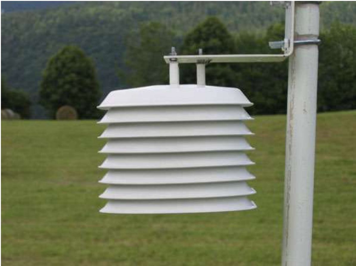
Figure 6.8: Example of a Radiation Screen in a Davis Weather Station [10]
