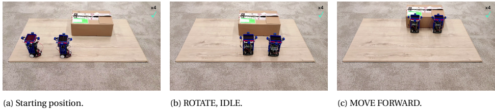
Figure 4.25: Successful collaborative task. Two robots push the carton box. Video is attached
