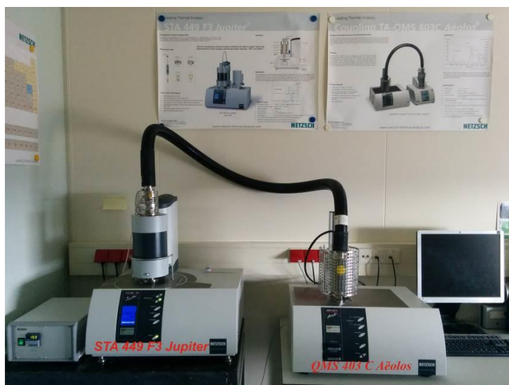
Figure 3-4 Netzsch STA 449 F3 Jupiter instrument used for thermogravimetric analysis
