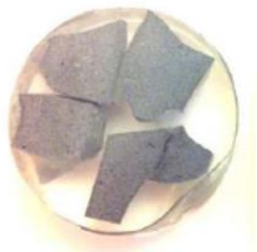
Figure 3-8 Polished sample for BSE-EDAX analysis (image from Yu[21])
