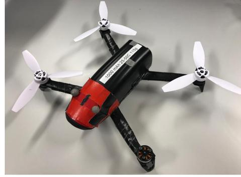
Fig. 6. Parrot Bebop 2 in 3 rotor configuration.
