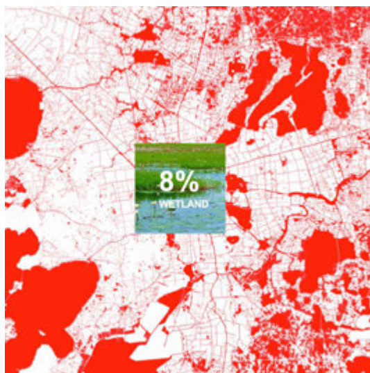
FIG. 3.60 8% of the land (excluding water surfaces) being wetland can both purify the run-off rainwater, and stock the storm water 规模为8%的陆地面积的湿地能够净化所有的雨水径流，同时在暴雨期承担蓄洪的作用
