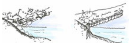
FIG. 3.165 Ecological Revetment Materials (from Left to Right): Soil and Plants, Biological Organic Materials.
