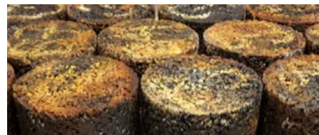
Figure 1. Corroded steel fibers in bituminous concrete samples
