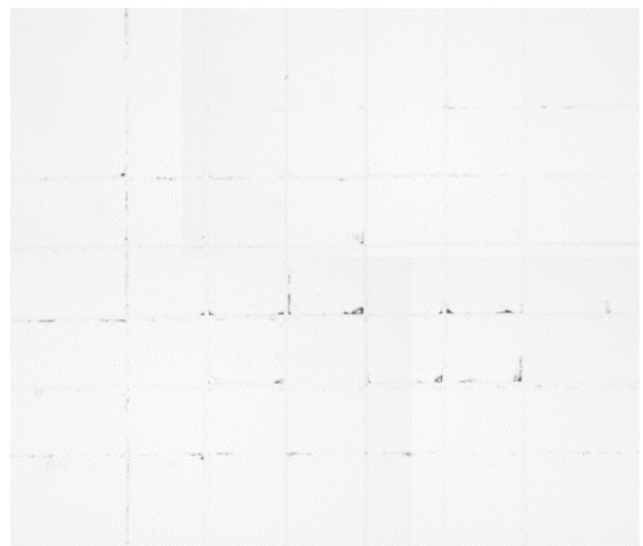
Figure C.27: Sample B2 (parylene on platinum) after peeling with 7.6 N/cm after 10 days in PBS at 55 °C.
