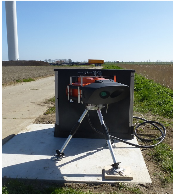
(b) Nacelle based LiDAR calibration facility
