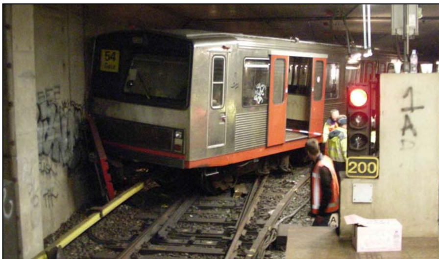
Figure 27. The derailed first coach of the metro train.
