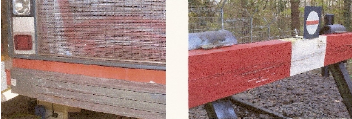
Figure 39. The red paint on the anti-climbers on the buffer beam and on the buffer stop
