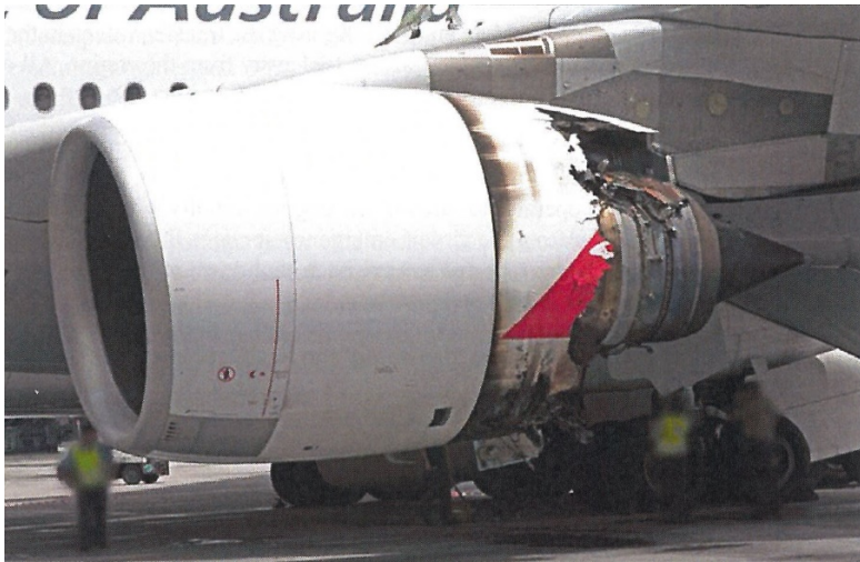
Figure 57. Damaged No. 2 engine (ATSB report)
