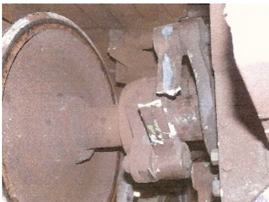
Figure 37. The disintegrated elastic transfer drive on the front axle
