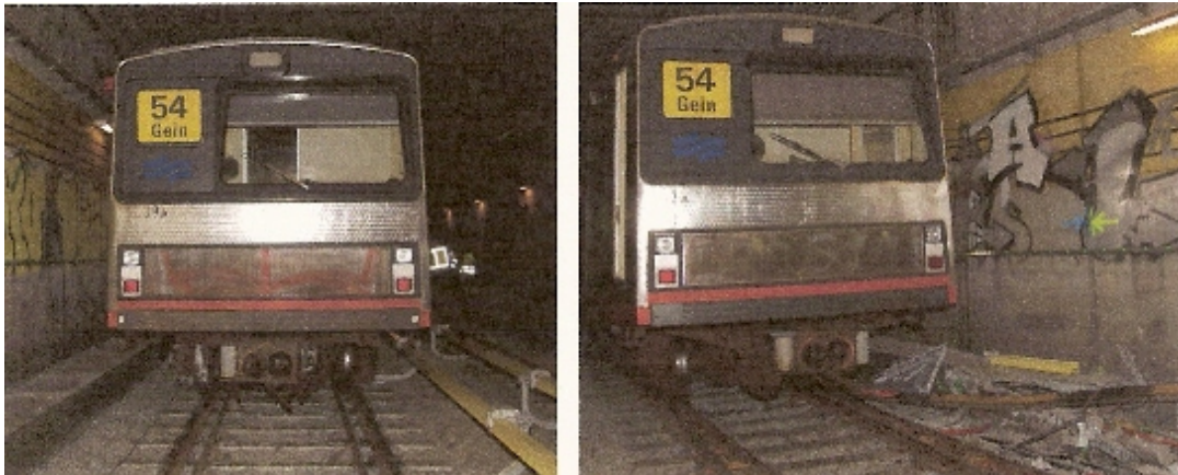
Figure 34. The derailed and damaged front (left) and rear (right) part of the metro
