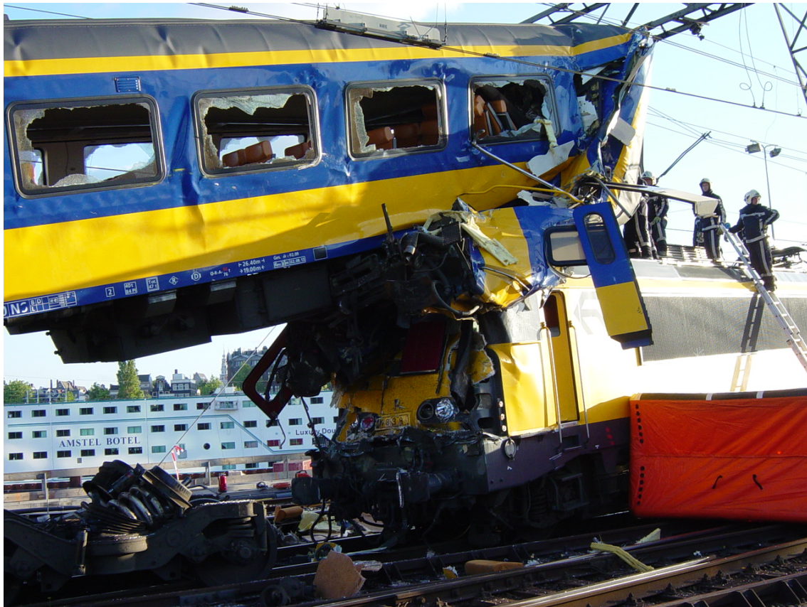
Figure 16: Low speed collision (<40 km/h) with serious consequences, because the coach broke its back; Amsterdam CS, 2004
