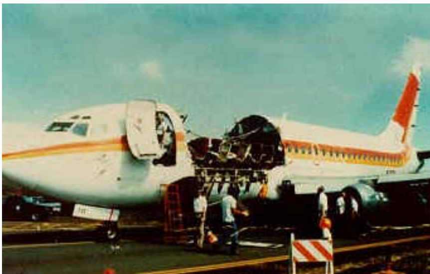
Figure 14: Aloha Airlines Boeing 737-200 after fatigue failure of the main fuselage, 1988
