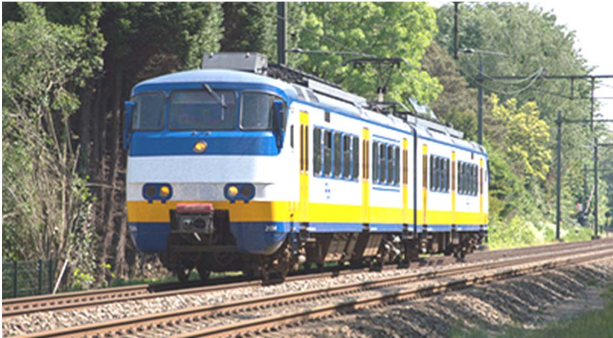
Figure 48. Sprinter type EMU class SGMm in two coach formation (SGMm-II).
