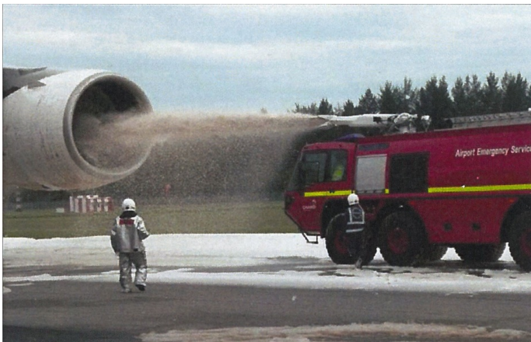
Figure 56. Fire-fighters drowning the runaway No. 1 engine with foam (ATSB report)
