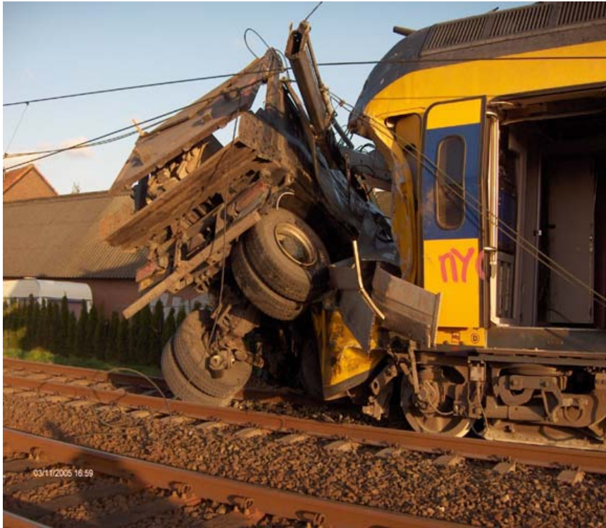
Figure 17: Collision between a Dutch Railways VIRM type electric multiple unit and a 40 ton loaded lorry, November 3, 2005. Although the damage to the train was severe, its resilient design prevented fatalities in the train.
