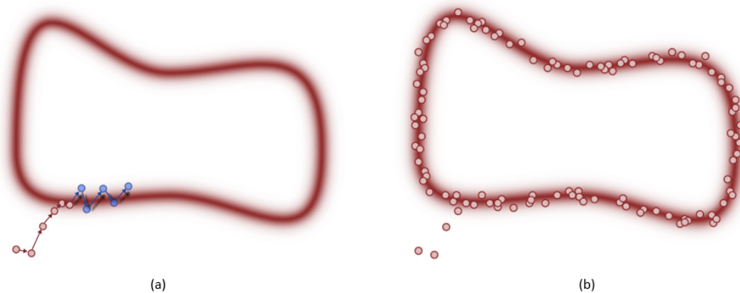
Figure 3.3: Graphical representation of how HMC and NUTS explore. (a) Random walks in parameter space (red) are combined with Hamiltonian trajectories in phase space (blue). Once the typical set (a thin surface with fuzzy boundaries) is reached, the Hamiltonian trajectory follows the gradient and stays close to the typical set. The trajectory ends when a new random state is proposed (not represented here). (b) Once the chain converges to the typical set, exploration is continued by taking samples (red) throughout the surface. (After Betancourt (2018) )
