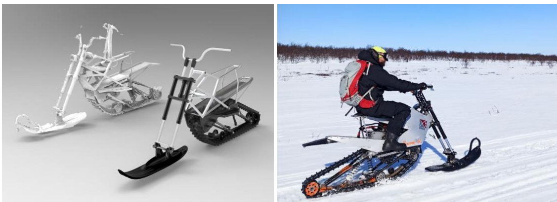
Figure 3. Left: 3D scan and 3D model of the snowbike, N. Korgin and N. Klyusov, 2021. Right: N. Korgin on the test drive in Kola tundra. Photo: A. Raeva, 2021.
