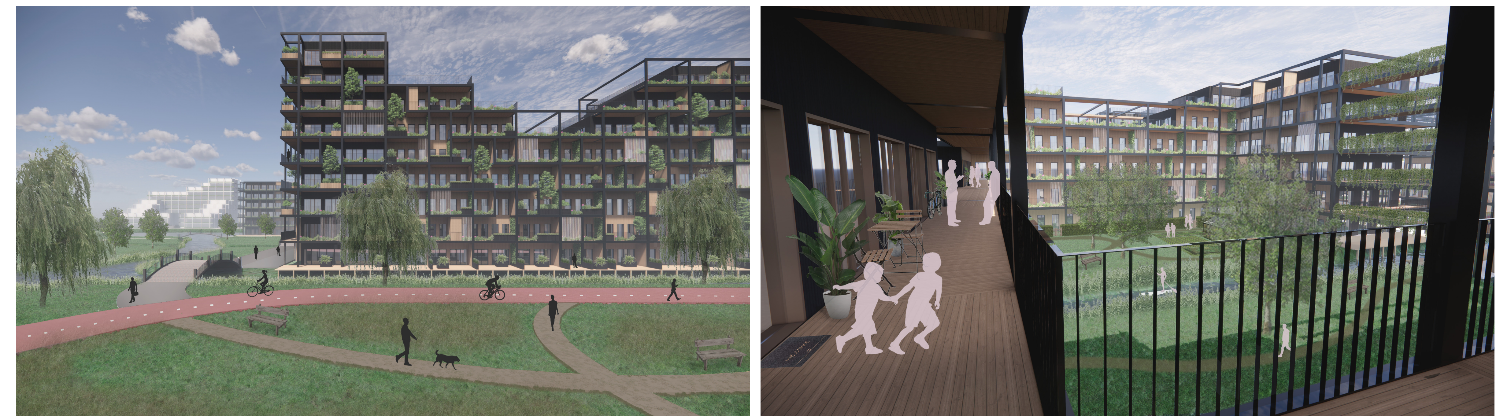
The smart support system is a fixed design with fixed dimensions, zones and materials. The corner has an open core which can be used for vertical access and services elements. The specific oversized dimensions of the support offers many possibilities for future alterations of the open building.
