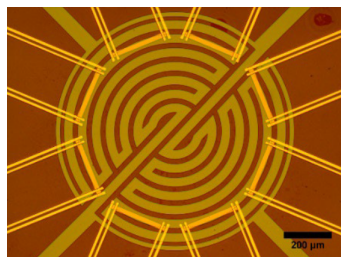
Figure 1.2: Array of 8 Graphene Strips integrated onto a Micro-Hotplate [4]
