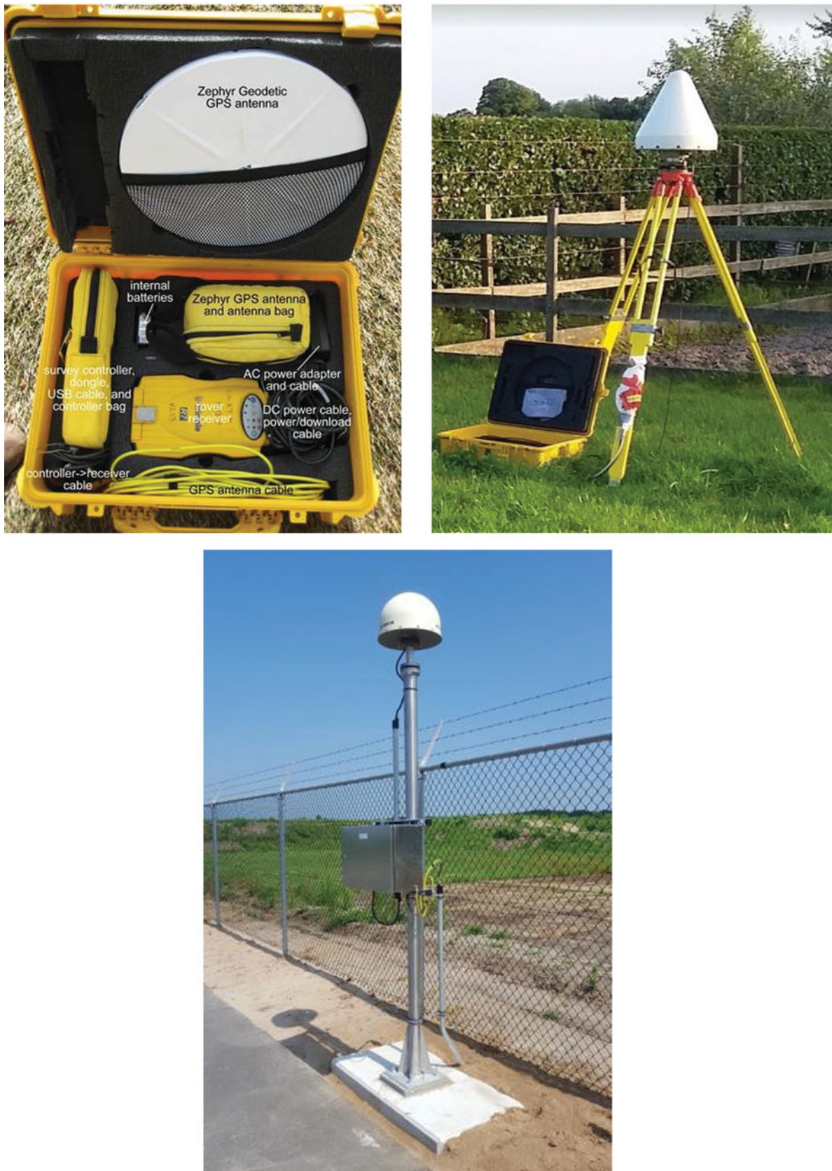
Fig. 12. Three examples of a geodetic receiver unit. On the left a campaign receiver and antenna in a case with all accessories (image courtesy UNAVCO), in the middle a typical field set-up with antenna on a tripod centred above a marker and battery-powered receiver in the waterproof case (data are stored on a flash card inside the receiver) (image TU Delft), and on the right a Continuous Operating Reference Station (CORS) from NAM, with receiver and data modem inside the cabinet (image courtesy 06-GPS).
