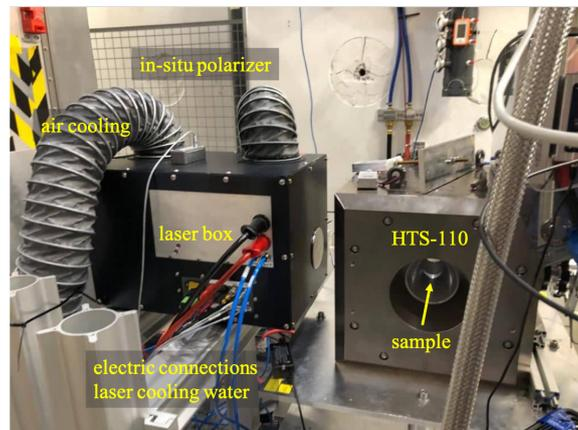
**Figure 2.** A photo of the KWS-1 analyzer installed on ZOOM at ISIS. The orientation is the same as in Fig. 2 with the sample magnet on the right and the *in-situ* polarized  $^3\text{He}$  polarization analyzer on the left. The sample area has ample space for the analyzer and the sample magnet is identical to that used on KWS-1, so ZOOM makes an optimal "sister-instrument" to KWS-1 for development work.
