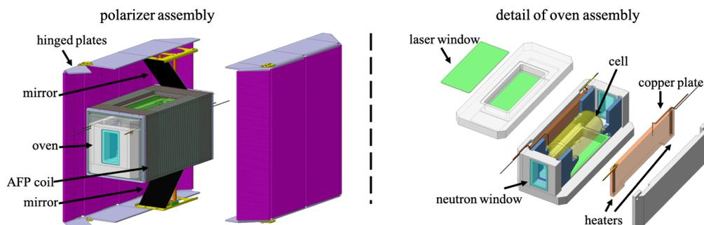
**Figure 4.** Expanded drawings showing detail of the new, double-angled opening+hinged magic box for POLI (left) and an expanded drawing of the oven detail which shows the heating plates to accommodate 4 stainless steel cartridge heaters and the up to 18 cm long  $^3\text{He}$  cell.
