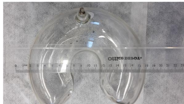
**Figure 6.** Photo of the PASTIS2 cell that was used for experiments on NEAT at HZB. This cell has a pressure of 1.5 bar and a 240 hour lifetime in laboratory conditions, it provided full polarization analysis coverage of the  $240^\circ$  horizontal and  $40^\circ$  vertical NEAT detector array.
