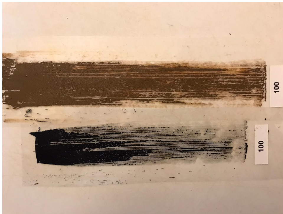
Figure 20: Two schematic reconstructions of the colours Brown under 1 and Black under that became streaky. When separated from melinex only small fragments came loose , unable to be used for tensile tests.
