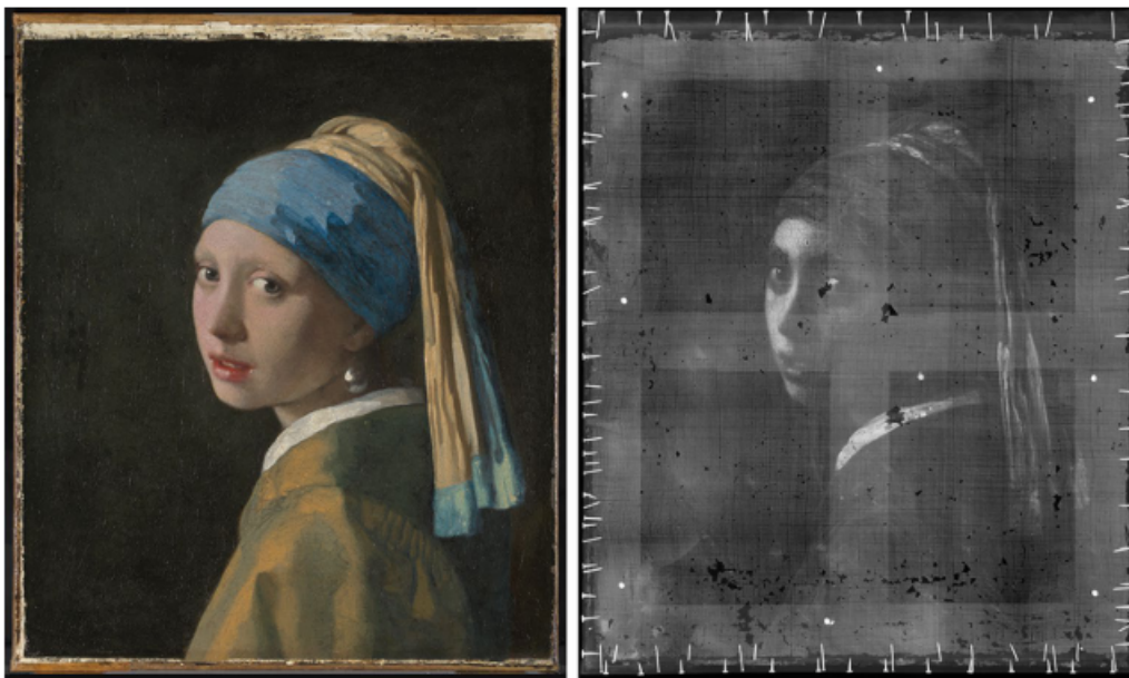
Figure 45: Left: Visible light photograph of Girl with a Pearl Earring . Right X-radiography photo of the same painting, visualising the wooden frame, canvas and nails. But, even more important, visualising black dots scattered over the painting. These black dots indicate the places where fragments of paint left the surface of the painting. In the middle a few bigger black spots can be seen, at the bottom an area of smaller dots. [11]
