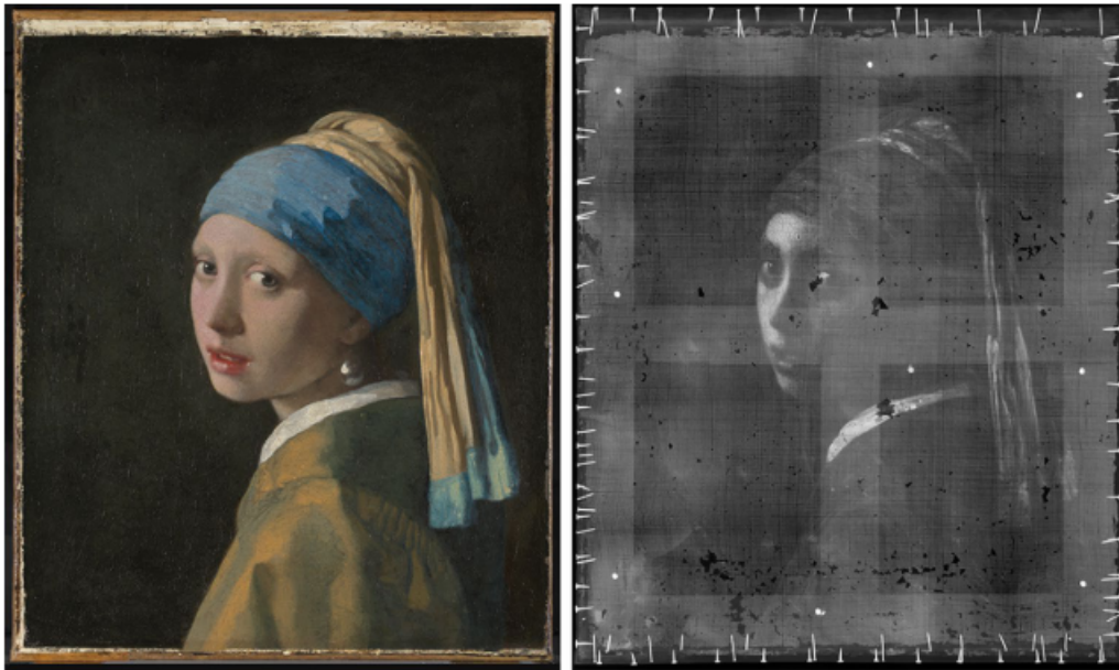
Figure 18: Left: Visible light photograph of Girl with a Pearl Earring . Right X-radiography photo of the same painting, visualising the wooden frame, canvas and nails. But, even more important, visualising black dots scattered over the painting. These black dots indicate the places where fragments of paint left the surface of the painting. In the middle a few bigger black spots can be seen, at the bottom an area of smaller dots. [11]
