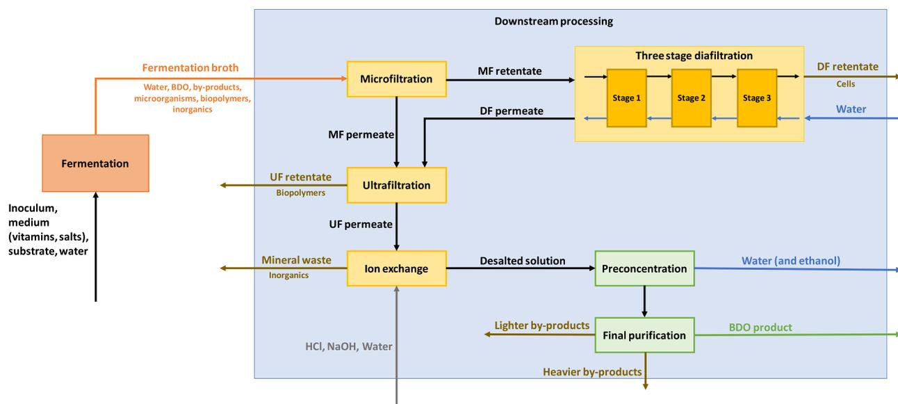
Fig. 1. Block flow diagram of the complete bioprocess (upstream and downstream), the focus of this work is on the preconcentration and final purification parts of the downstream processing.
