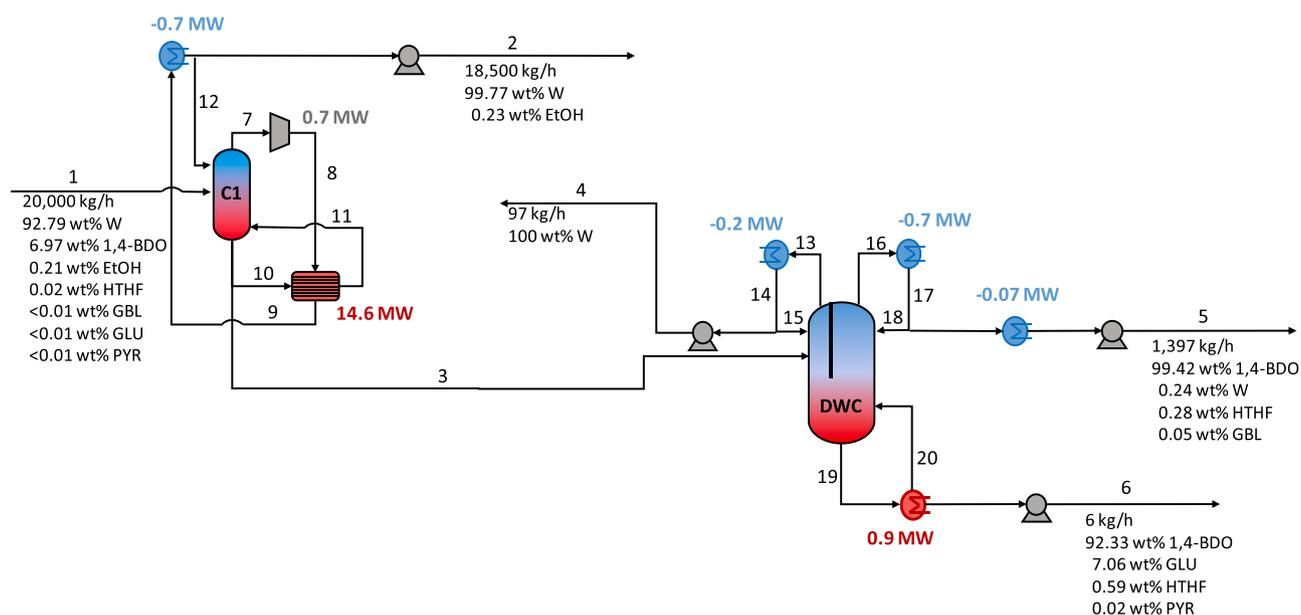
**Fig. 3.** Downstream process for the final purification of 1,4-BDO after fermentation (case 1–4), conditions and compositions of the numbered process streams are given in Table 3 (abbreviations: W – water, 1,4-BDO – 1,4-butanediol, EtOH – ethanol, GBL – gamma butyrolactate, HTHF – 2-(4-hydroxybutoxy)-THF, PYR – 2-pyrrolidone and GLU – glucose).
