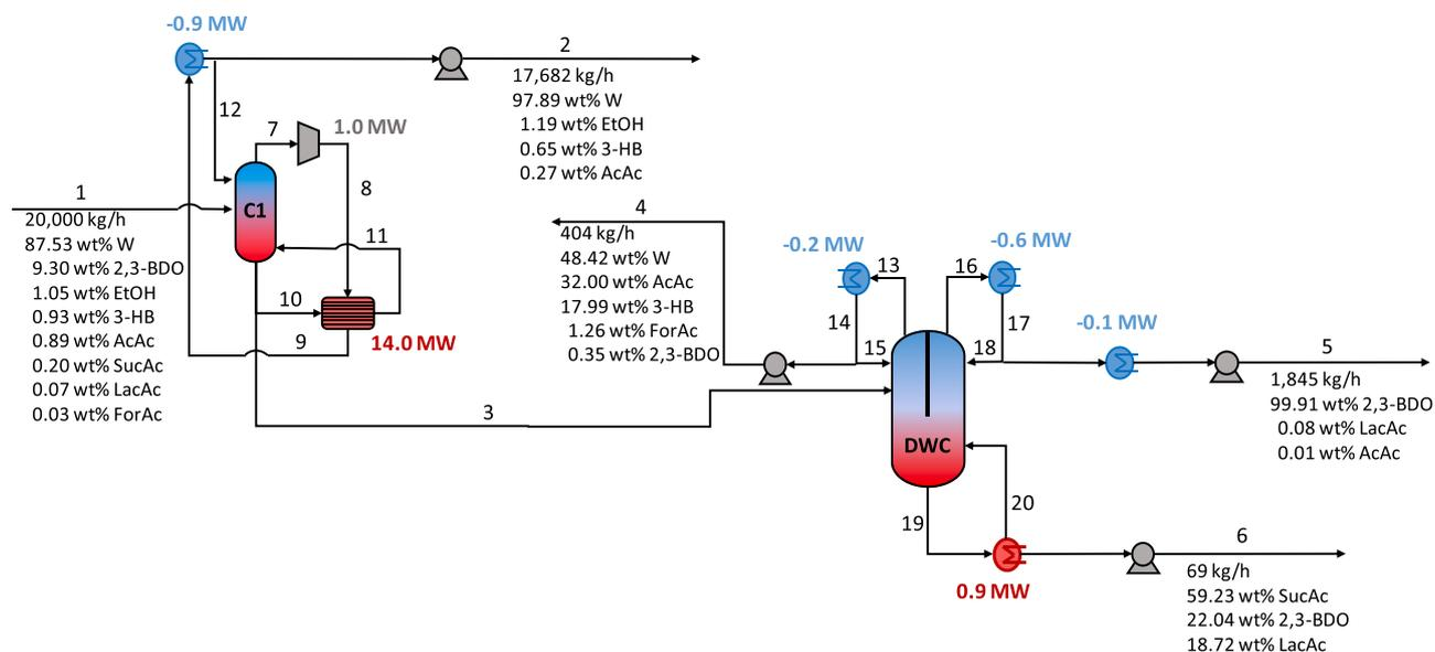
**Fig. 2.** Downstream process for the final purification of 2,3-BDO after fermentation (case 2–3), conditions and compositions of the numbered process streams are given in Table 2 (abbreviations: W – water, 2,3-BDO – 2,3-butanediol, EtOH – ethanol, ForAc – formic acid, AcAc – acetic acid, LacAc – lactic acid, SucAc – succinic acid and 3-HB – 3-hydroxy-2-butanone).
