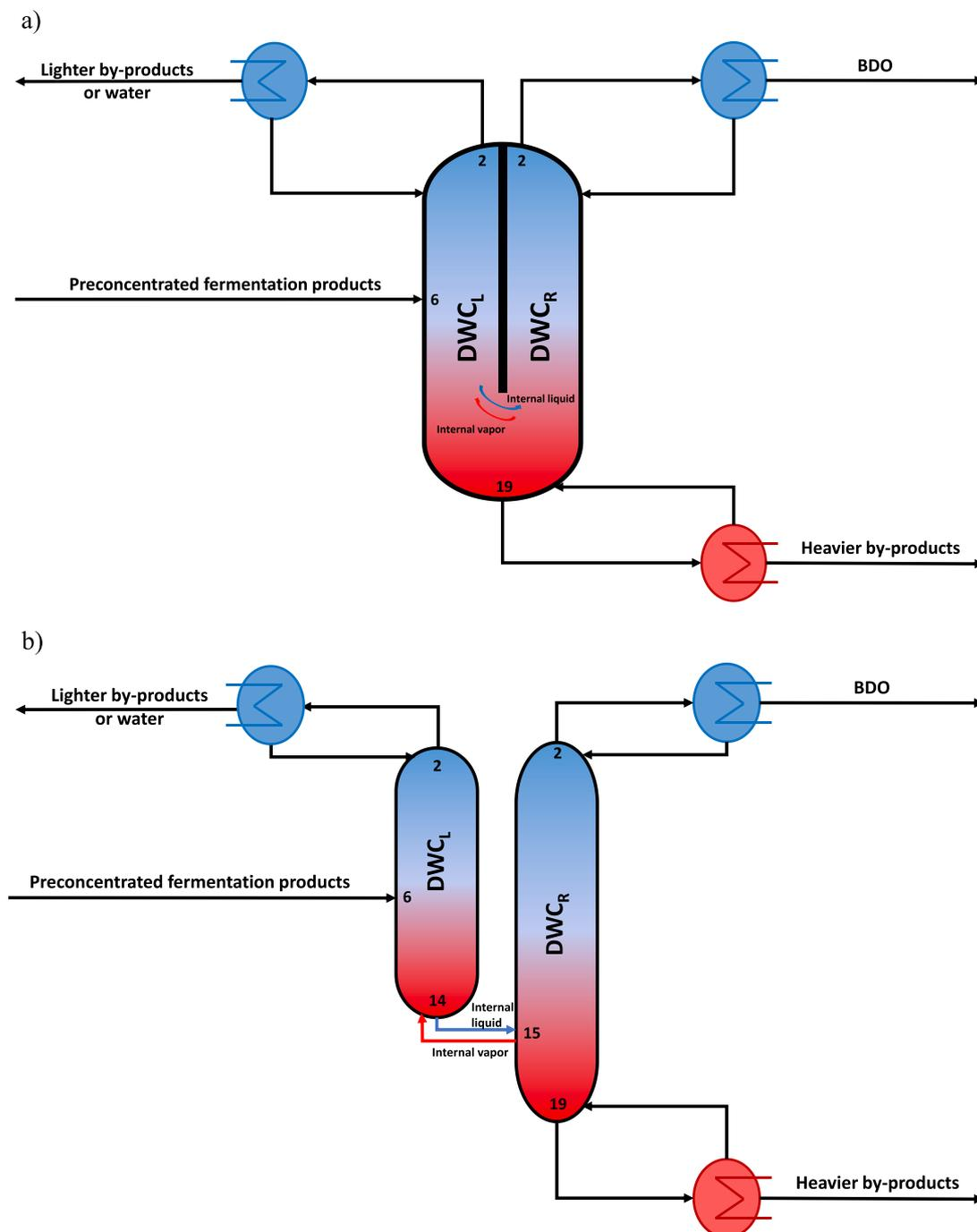
Fig. 5. DWC design (a) and the equivalent sequence of distillation columns (b) - the numbers in the column indicate the column tray number.
