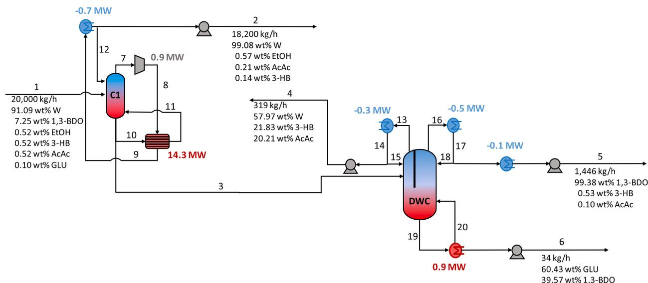
Fig. 4. Downstream process for the final purification of 1,3-BDO after fermentation (case 1–3), conditions and compositions of the numbered process streams are given in Table 4 (abbreviations: W – water, 1,3-BDO – 1,3-butanediol, EtOH – ethanol, AcAc – acetic acid, 4-HB – 4-hydroxy-2-butanone and GLU – glucose).
