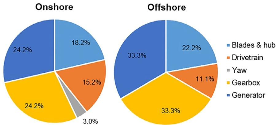
**Fig. 5** Downtime distribution among the main WT assembly/components for 14 onshore and 4 offshore reliability databases (Dao et al., 2019). From Dao C, Kazemtabrizi B, and Crabtree C (2019) Wind turbine reliability data review and impacts on levelised cost of energy. *Wind Energy* 22: 1848–1871.
