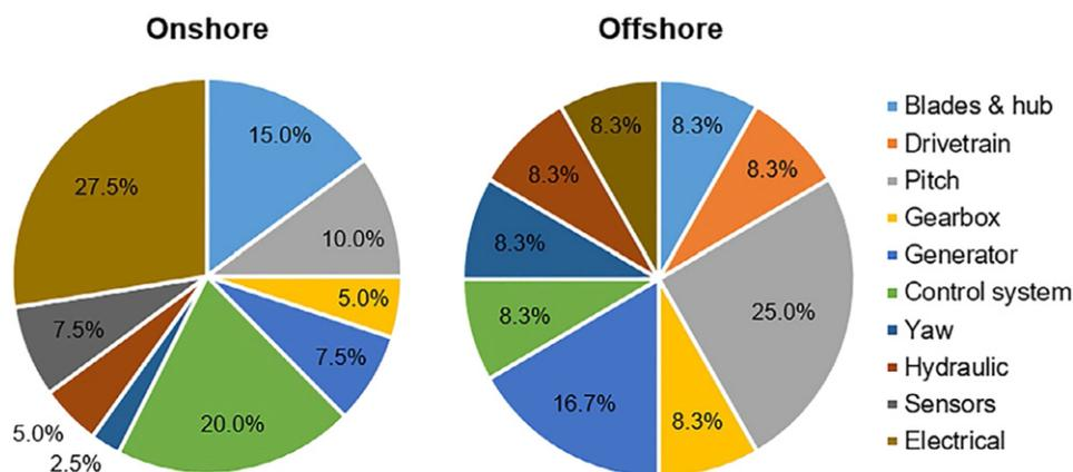
Fig. 4 Failure rate distribution among the main WT components for 14 onshore and 4 offshore reliability databases (Dao et al., 2019). From Dao C, Kazemtabrizi B, and Crabtree C (2019) Wind turbine reliability data review and impacts on levelised cost of energy. *Wind Energy*, 22: 1848–1871.
