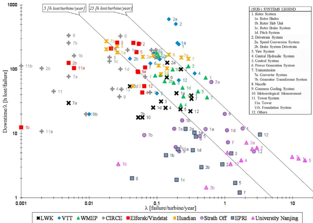
**Fig. 6** Failure rate vs. downtime per component according to Cevasco et al. (2021). From Cevasco D, Koukoura S, and Kolios AJ (2021) Reliability, availability, maintainability data review for the identification of trends in offshore wind energy applications. *Renewable and Sustainable Energy Reviews* 136: 110414.
