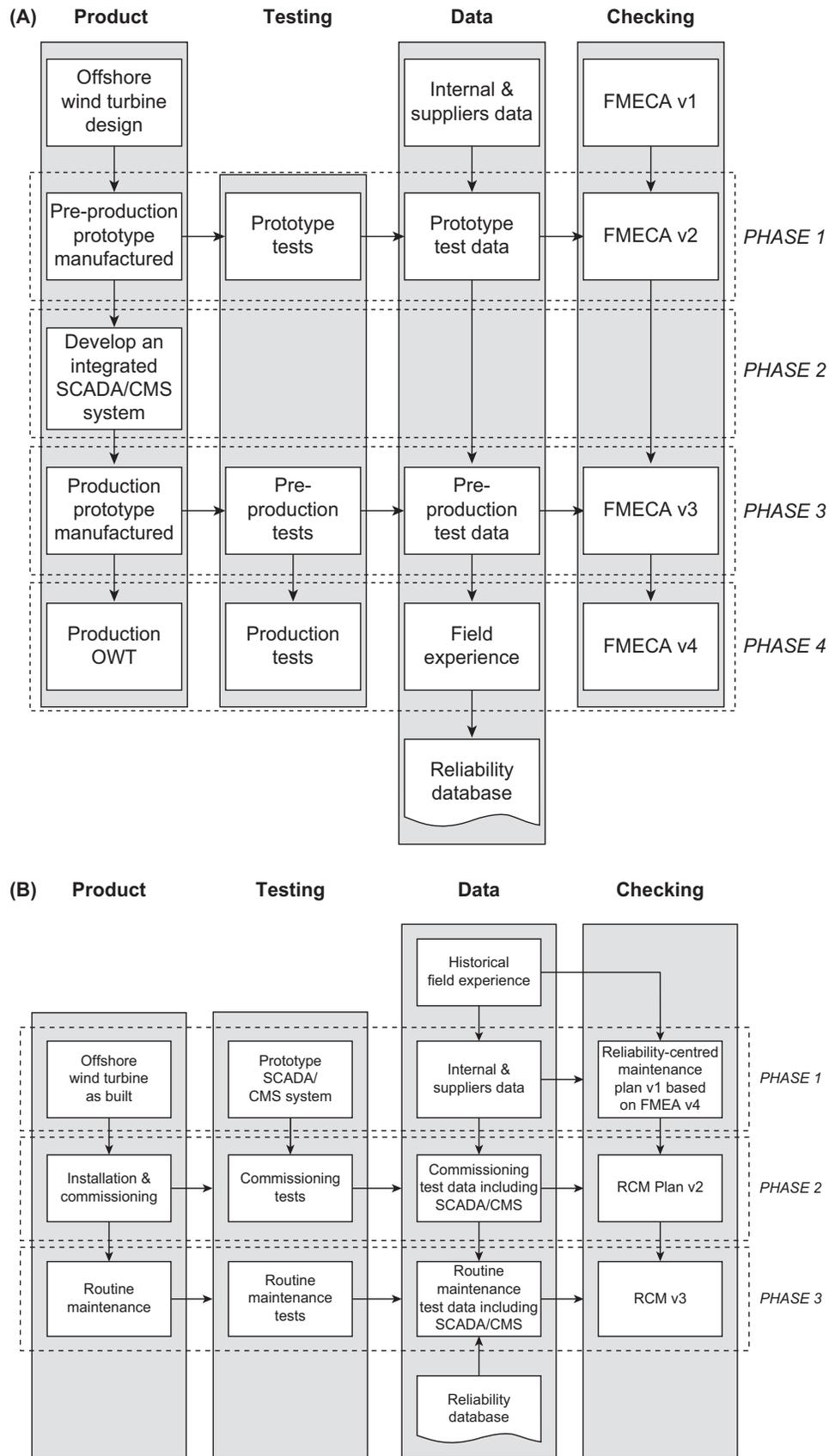
**Fig. 8** Proposals to use of FMEA and Reliability-Centered Maintenance (RCM) as Review Tools during Offshore WT Design and Manufacture for improved WF O&M outcomes (Tavner, 2021). (A) FMEA as a Design Review Tool; (B) FMEA and RCM together as an O&M Review Tool. From Tavner PJ (2021) Offshore Wind Power - Reliability Availability and Maintenance, 2nd edn. London, UK: The Institution of Engineering and Technology.
