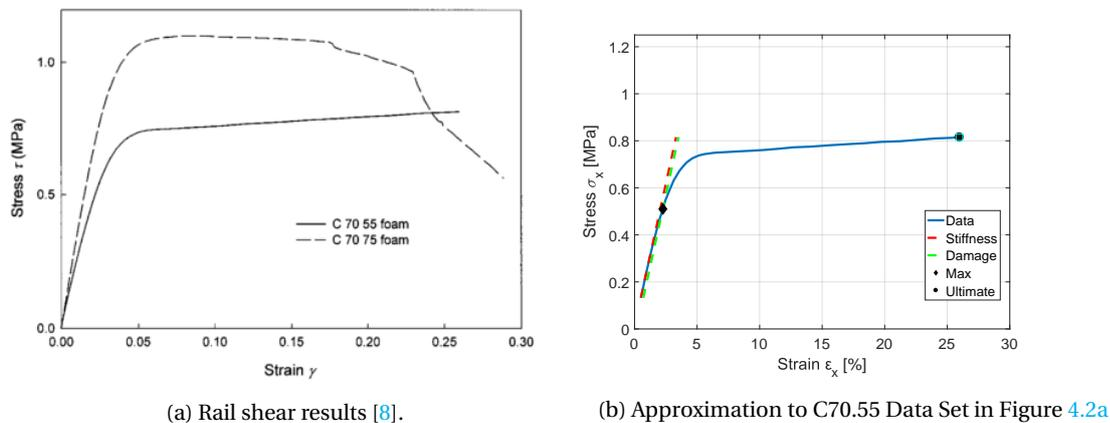
Figure 4.2: Rail shear stress-strain curves from research by Berthelot et al. [8].
