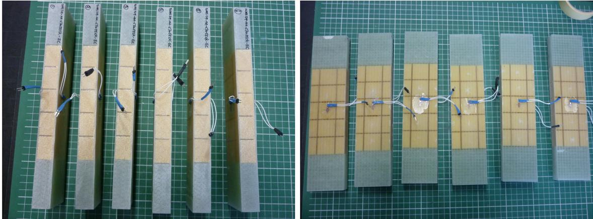
(a) Side view of EC test specimens.
