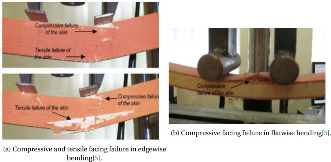
Figure 3.13: Core facing failure in flatwise and edgewise bending[5].
