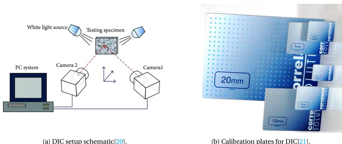
(a) DIC setup schematic[20].
