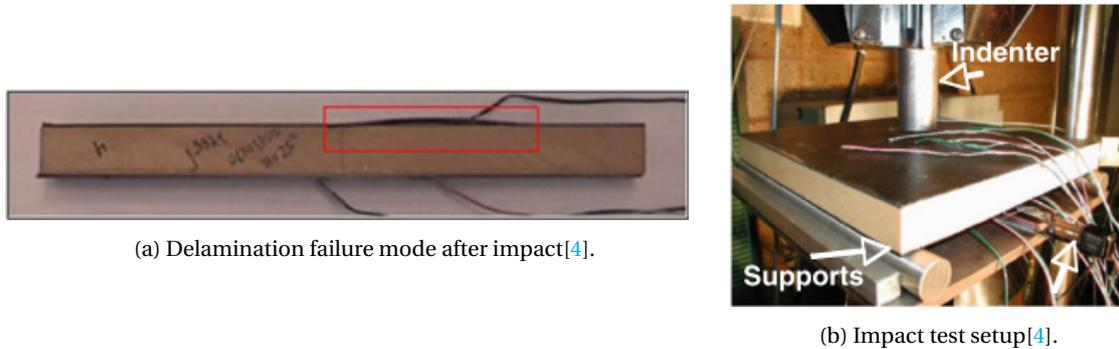
Figure 3.12: Impact induced delamination and test setup[4].
