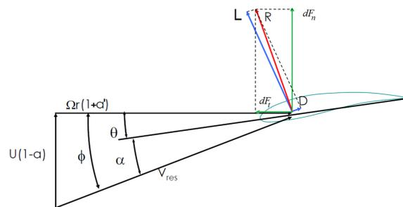
Figure 3.2: Velocity Triangle; Schematising the apparent wind experienced by a section of a wind turbine blade.
