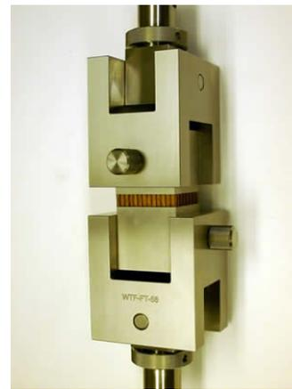
(b) Example of a 90 degree cardanian support fixture[22].
