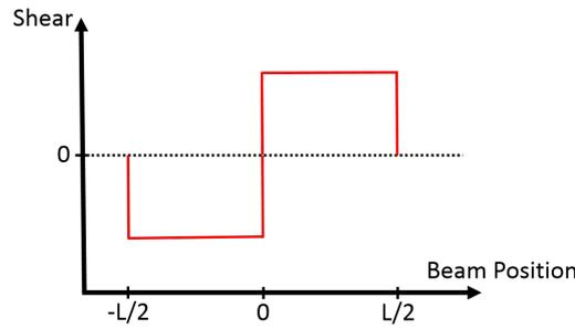
Figure 5.13: Three point bending shear diagram.
