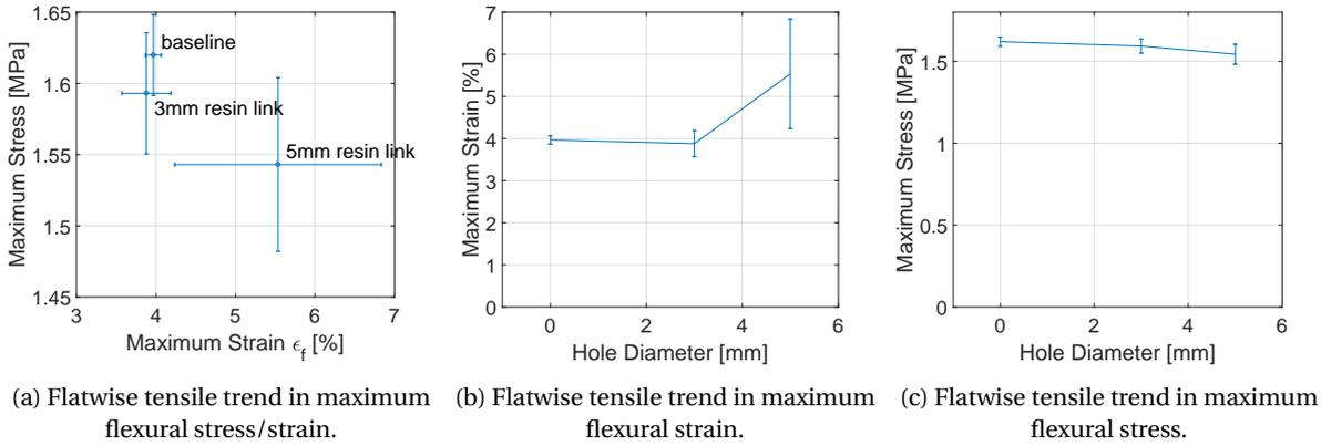
Figure 5.6: Flatwise tensile trends of benchmark and 3mm & 5mm resin link cases.
