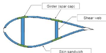
Figure 3.3: Typical wind turbine blade cross-section[2].
