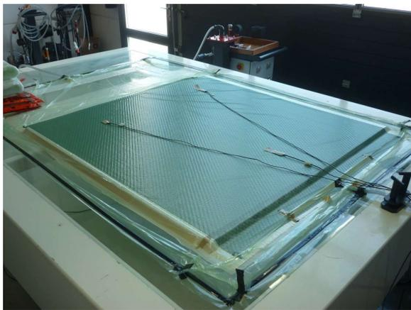
(c) Thermocouples attached to the sandwich plate.
