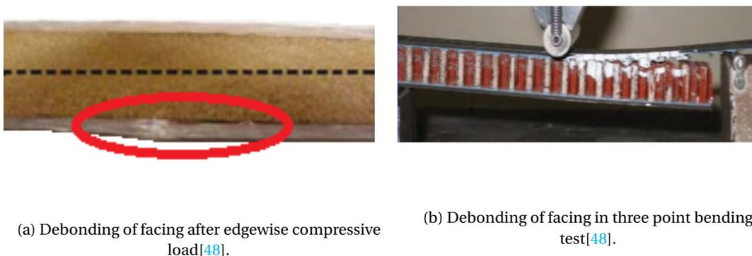
Figure 3.14: Debonding of facings in edgewise compression and three point bending loading.
