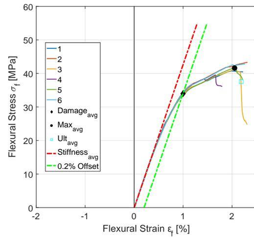
(b) TPB sandwich SD flexural stress-strain curve
