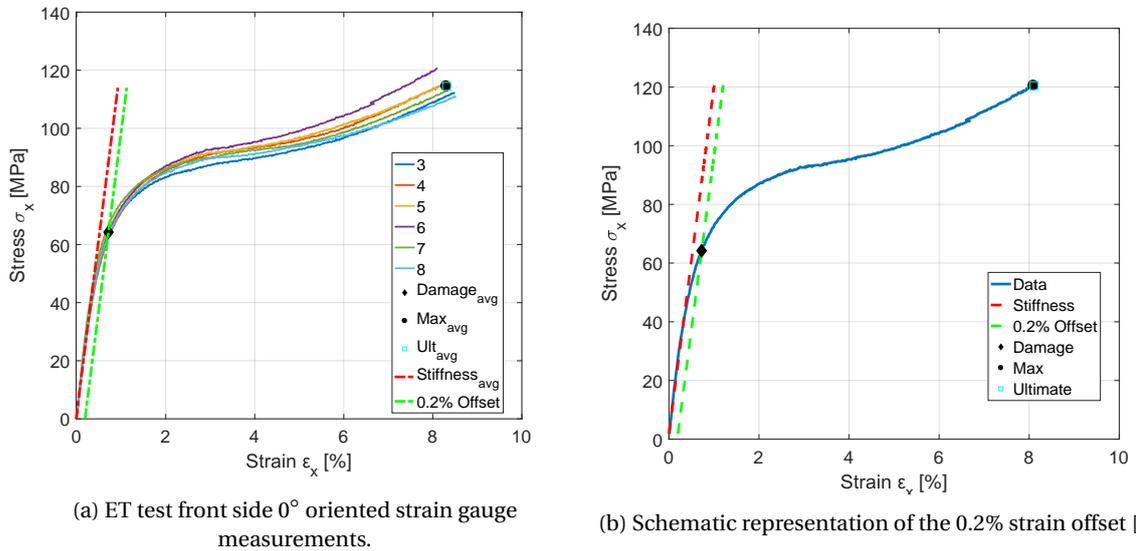
Figure A.2: Front side measurements and computed important parameters.
