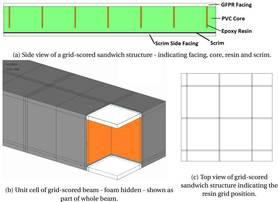
Figure 2.1: Normal "benchmark" grid-scored core sandwich structure.
