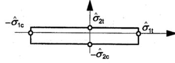
Figure 3.9: Maximum stress failure criterion for a brittle material[3].
