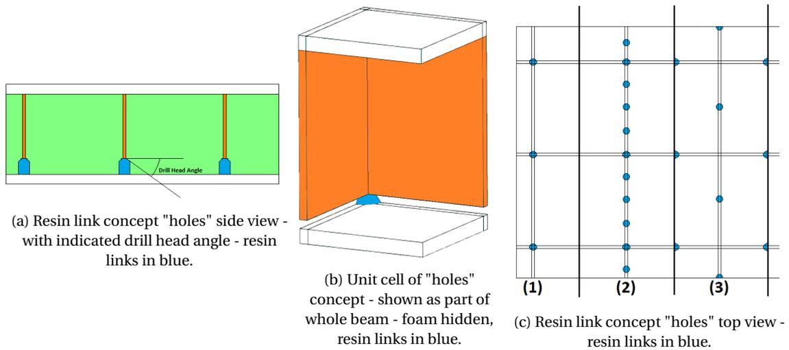
Figure 2.3: Concept "holes" sandwich structure - side and top view - resin links in blue.
