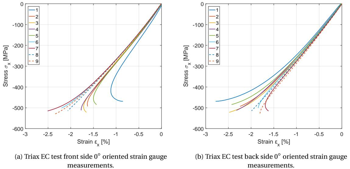
Figure A.7:  $0^\circ$  oriented strain gauge measurements for the edgewise tensile test of the biax and triax coupons.
