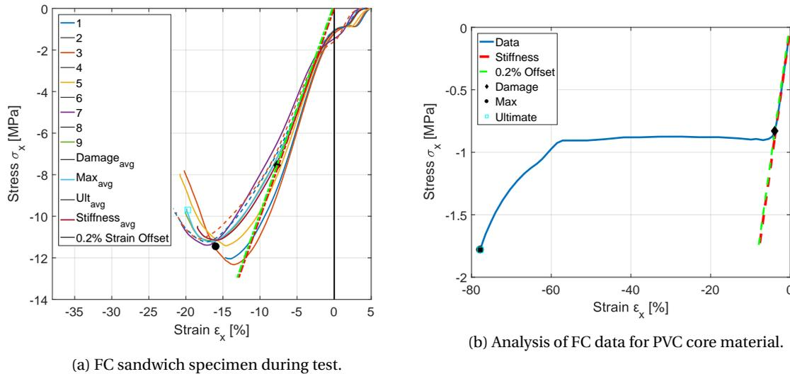
Figure A.27: Analysis of sandwich and PVC core FC tests.
