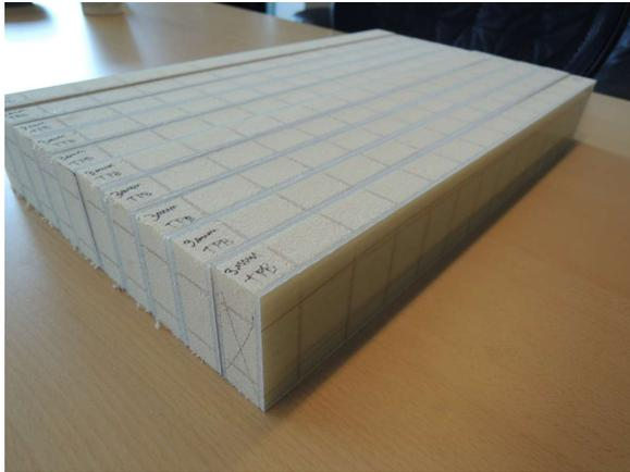
(a) 3mm TPB specimens showing a small deviation in widths.
