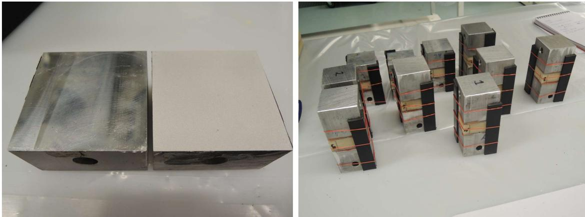
(a) Loading blocks before (left) and after (right) sandblasting.
