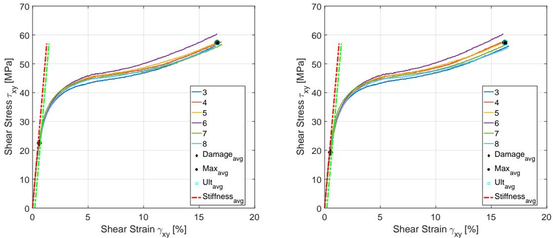
(a) ET test shear stress vs shear strain - front facing. (b) ET test shear stress vs shear strain - back facing.
