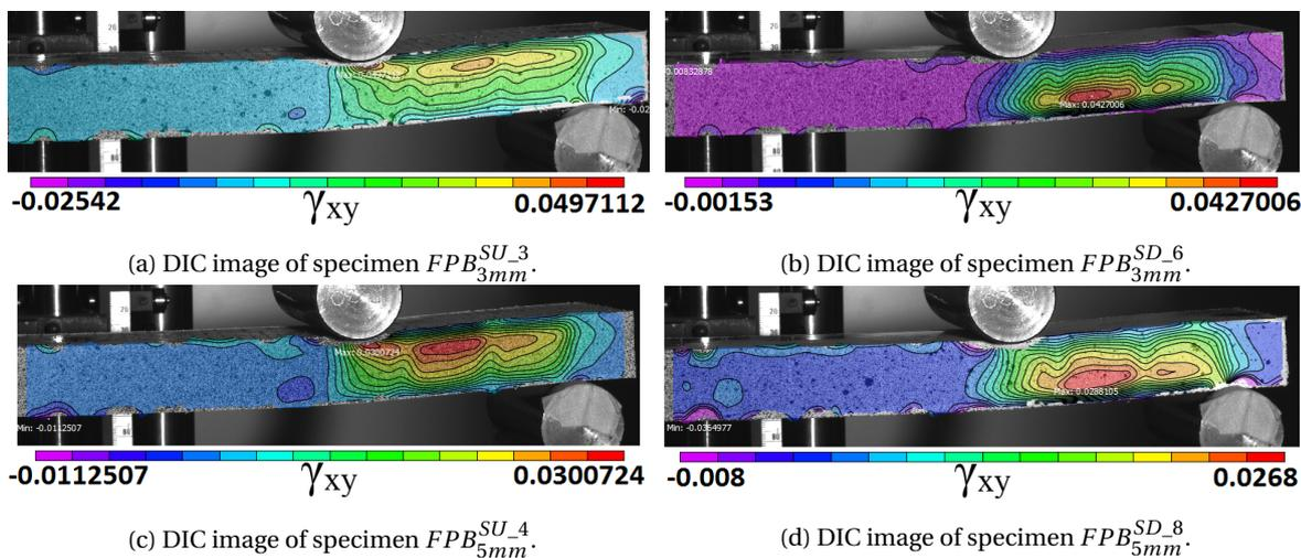
Figure 5.22: DIC Images for the FPB Test of the 3mm and 5mm resin link specimens. Images taken right before failure.
