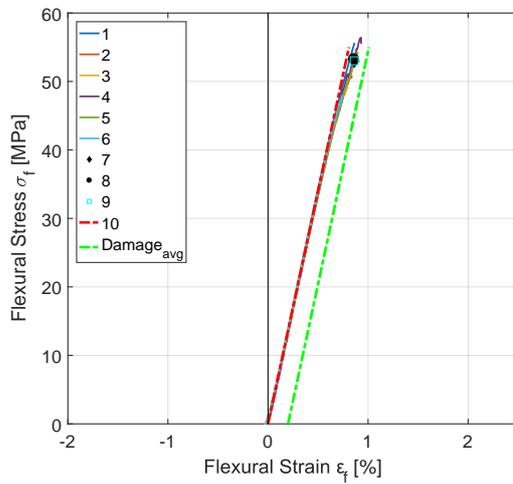
(a) TPB sandwich SU flexural stress-strain curve
