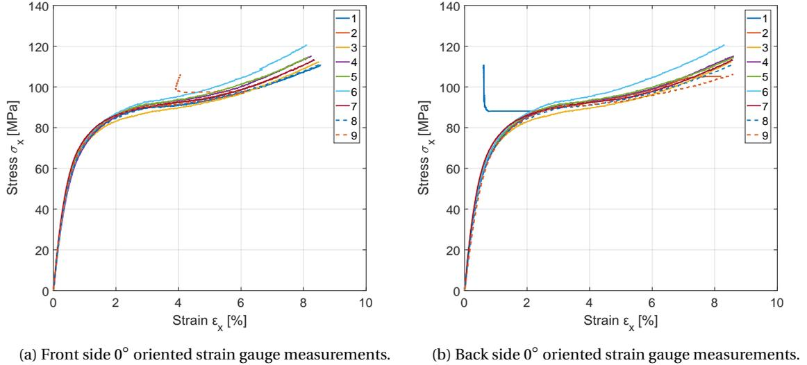
Figure A.1:  $0^\circ$  oriented strain gauge measurements for the edgewise tensile test of the biax coupons.
