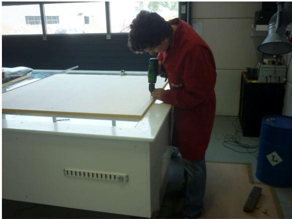
(a) Drilling of holes in the 1220x1220mm PVC core plate.
