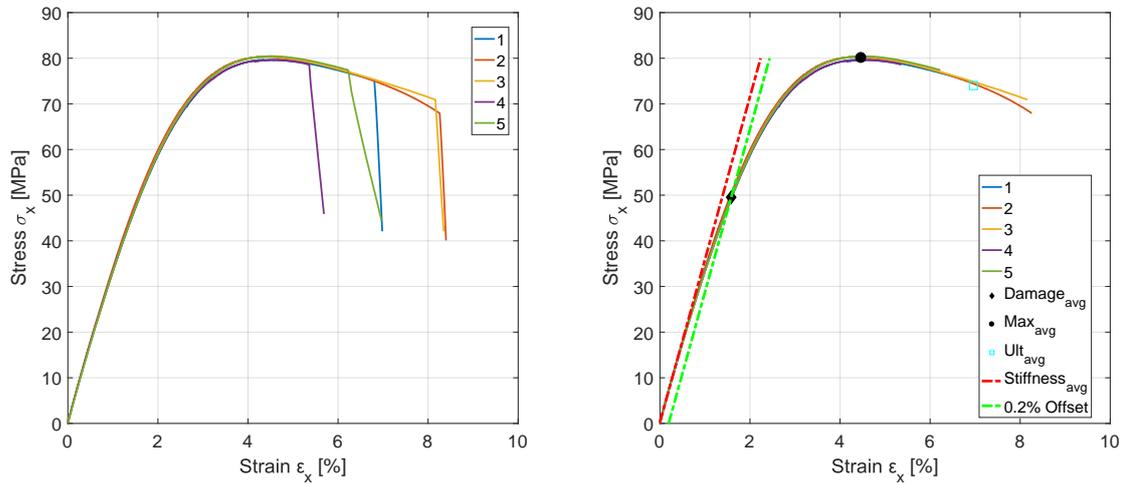
(a) Resin Y - Stress-strain curves for 5 tested specimens.
