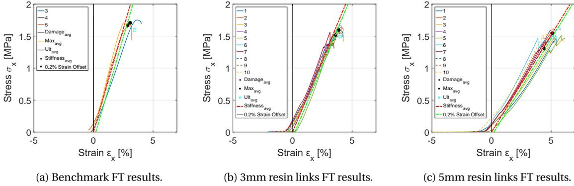
Figure 5.5: Stress-strain graphs of benchmark, 3mm and 5mm resin link specimens for flatwise tension
