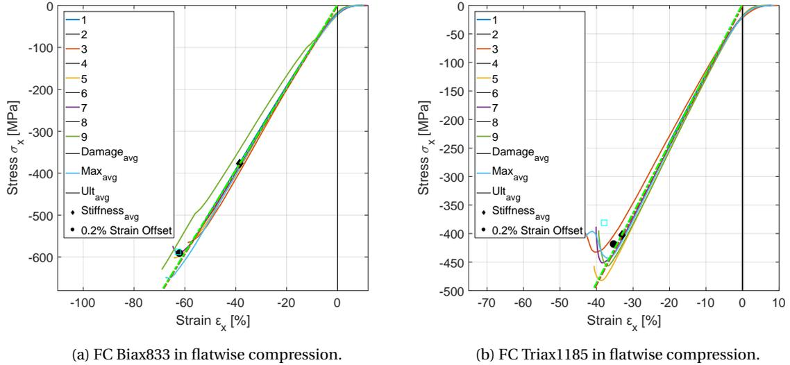
Figure A.9: Stress-strain curves for biax and triax specimens loaded in flatwise compression.
