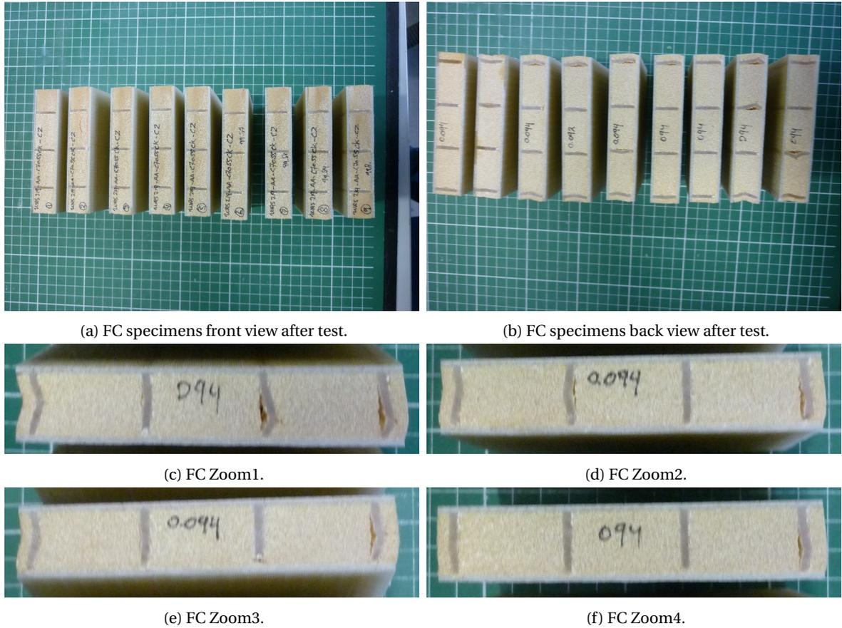
Figure A.26: FC specimens after testing showing different damage modes.
