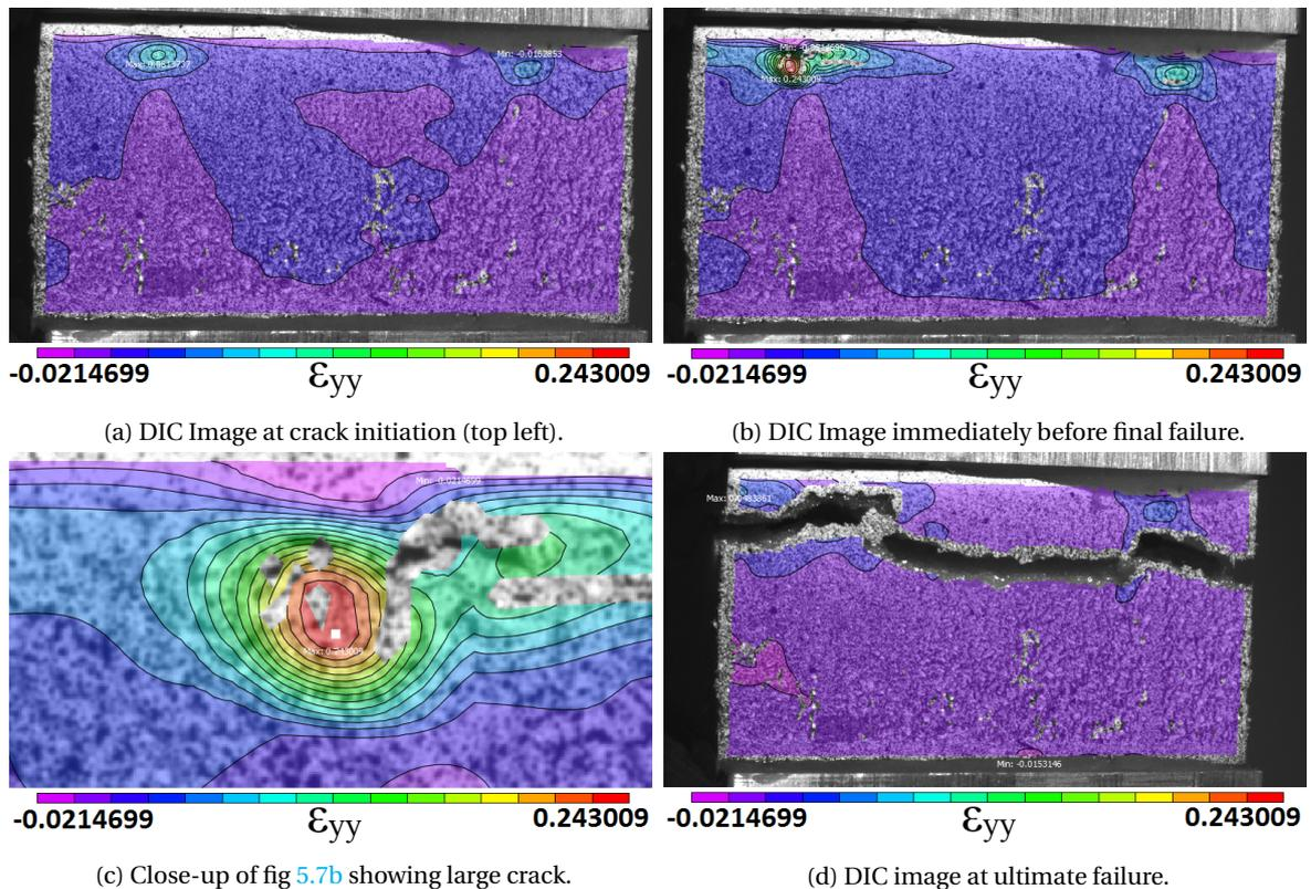
Figure 5.7: DIC images for the flatwise tensile test of the 3mm resin link specimens.
