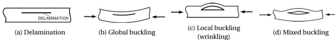
Figure 3.16: Induced delamination and possible subsequent buckling failure modes (Figures[6]).
