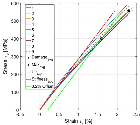
(a) ET test stress vs strain - triax front facing.
