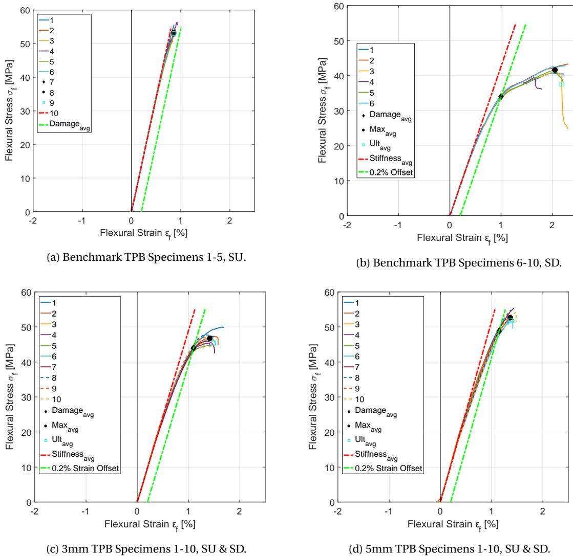
Figure 5.14: Stress-strain graphs for three point bending specimens for benchmark and 3mm and 5mm resin links.
