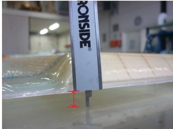
(b) Close-up of measuring the warp = distance measured with calipers between table and sandwich plate.
