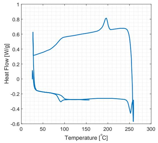
(b) Heat flow measurement of post-cured sample.
