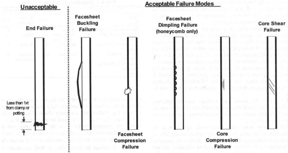
Figure A.15: Acceptable and unacceptable failure modes for ASTM C364.
