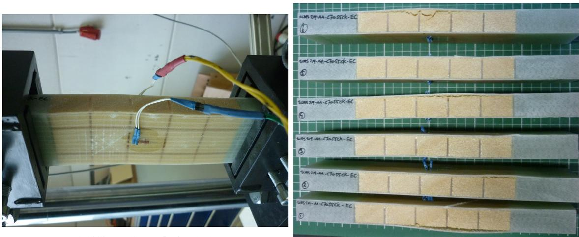
(a) EC specimen during test.
