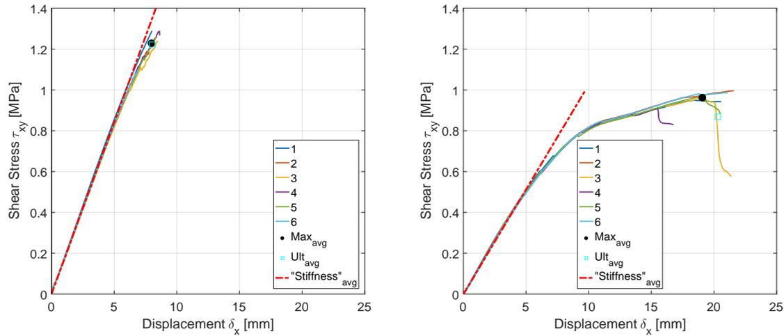
(a) TPB sandwich SU shear stress-displacement curve (b) TPB sandwich SD shear stress-displacement curve
