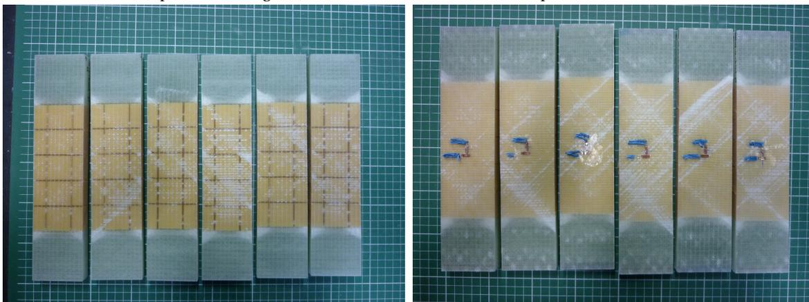
(c) ET specimens front view after test.
