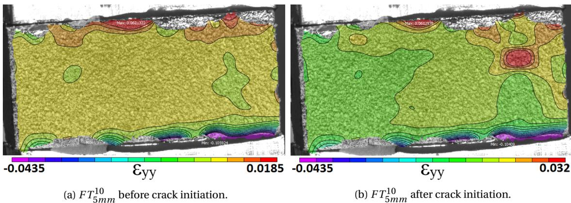
Figure 5.8:  $FT_{5mm}^{10}$  before (left) and after (right) crack initiation.
