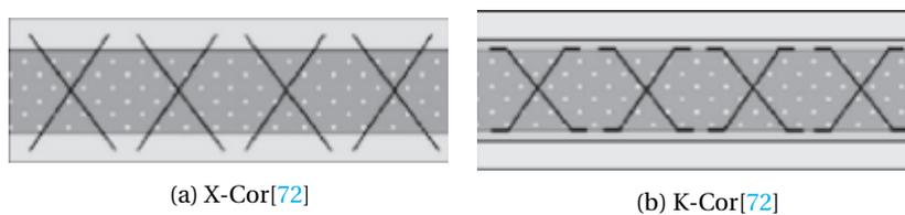
Figure 3.21: Core materials with strong fibre pin reinforcements through the thickness
