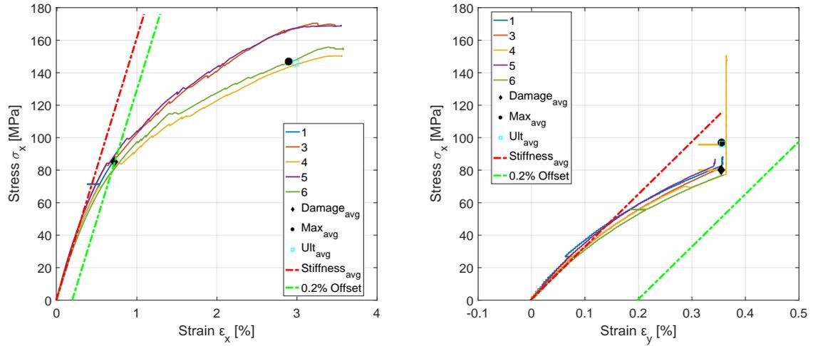
(a) Stress-strain curves using  $0^\circ$  oriented strain gauges. (b) Stress-strain curves using  $90^\circ$  oriented strain gauges.
