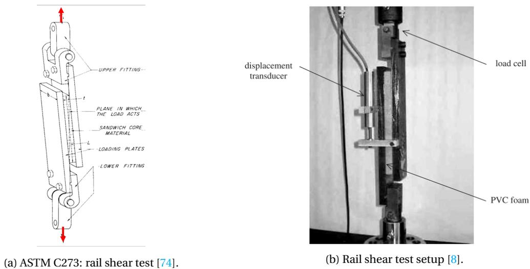
Figure 4.1: Rail shear test type schematic and test setup picture.
