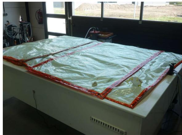
(d) Insulation of the sandwich plate during infusion.
