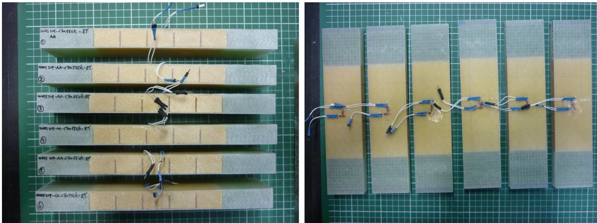
(a) Side view of ET test specimens.
