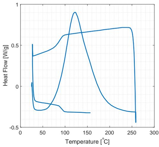
(a) Heat flow measurement of pre-cured sample.
