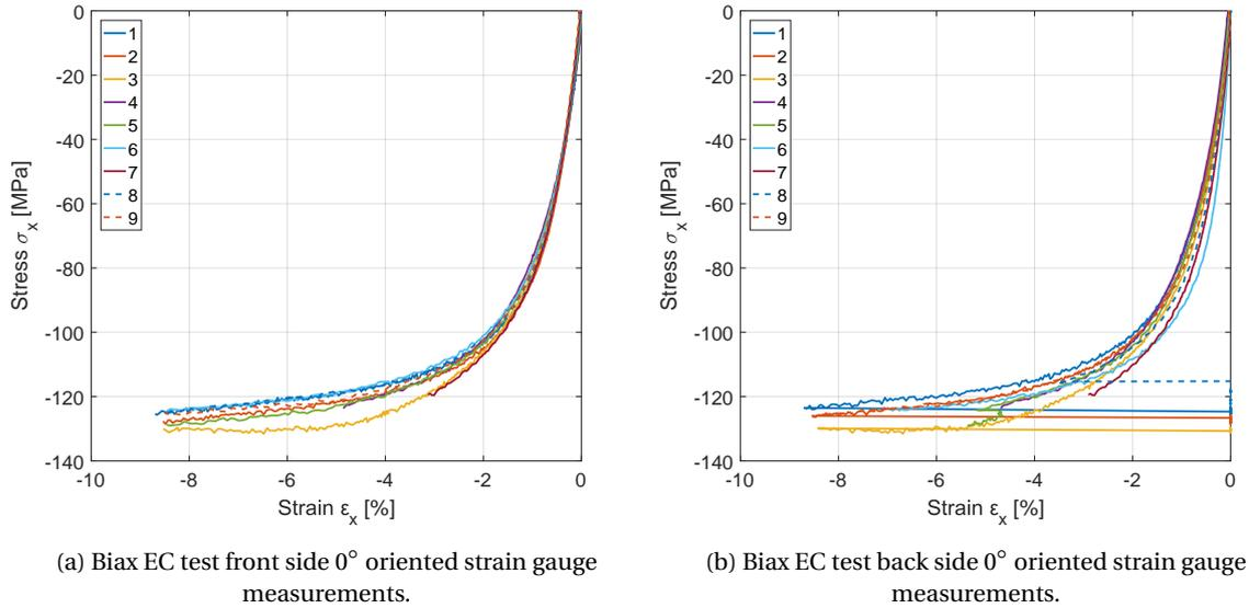
Figure A.6:  $0^\circ$  oriented strain gauge measurements for the edgewise tensile test of the biax coupons.
