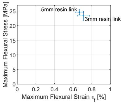
(a) FPB trend in maximum flexural stress/strain.
