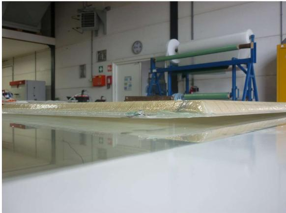
(a) Close-up of the plate showing warp. There is a clear gap between the sandwich plate and the table.
