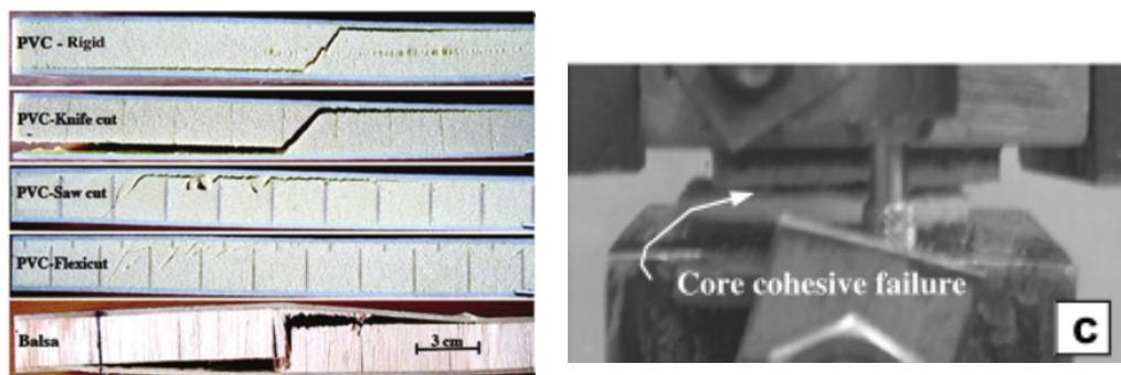
(a) Core failure in four point bending test for different core types[15].
