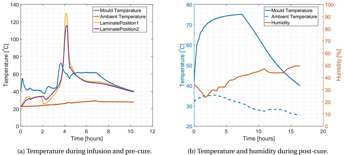
Figure 2.14: Temperature during pre- and post-cure.
