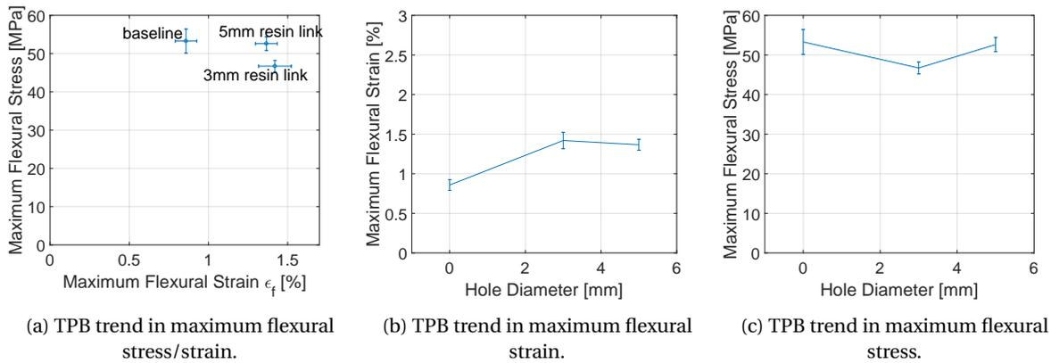
Figure 5.16: TPB trends of benchmark and 3mm &amp; 5mm resin link cases.
