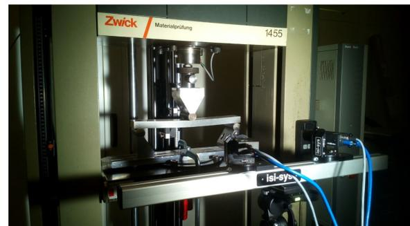
(b) TPB test setup.
