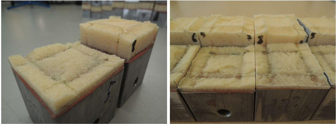
(a) Close-up of 3mm flatwise tension specimen.
