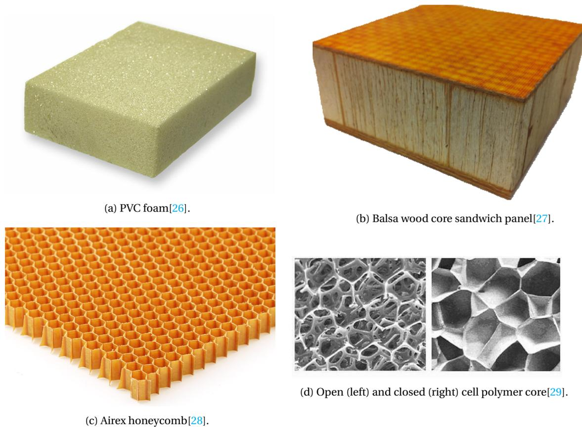
Figure 3.7: Different core types used for composite sandwich construction.
