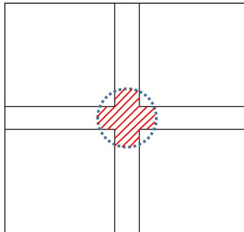
Figure 2.5: Top view of resin link structure showing overlap in resin link and resin bridge.
