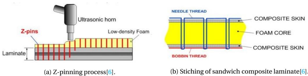
Figure 3.20: Core materials with reinforcements through the thickness.
