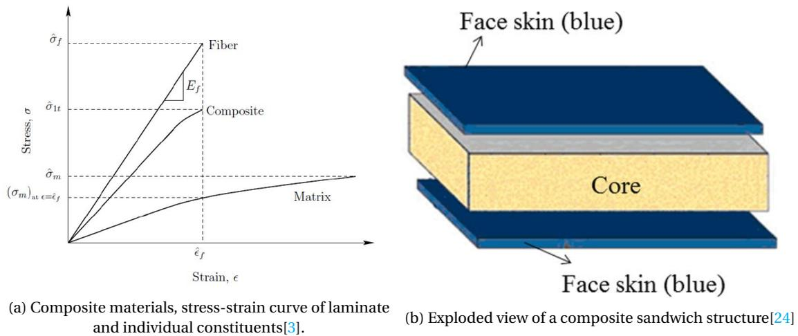
Figure 3.5: Composite - individual properties and composite sandwich layout.
