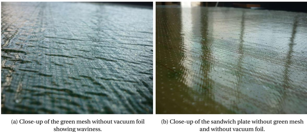
Figure 2.15: Inspection of the sandwich plate after pre-cure; close-up.
