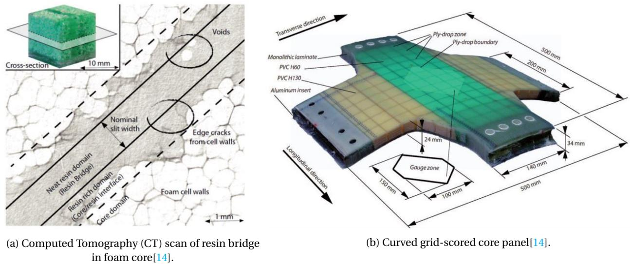
Figure 3.18: Grid-scored core structures
