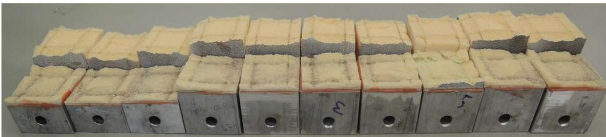
Figure 5.1: Flatwise tension specimens of sandwich structures with 3mm resin links after test.
