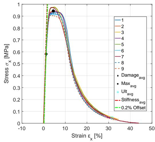
Figure A.28: Sxz sandwich shear stress-shear strain curve.
