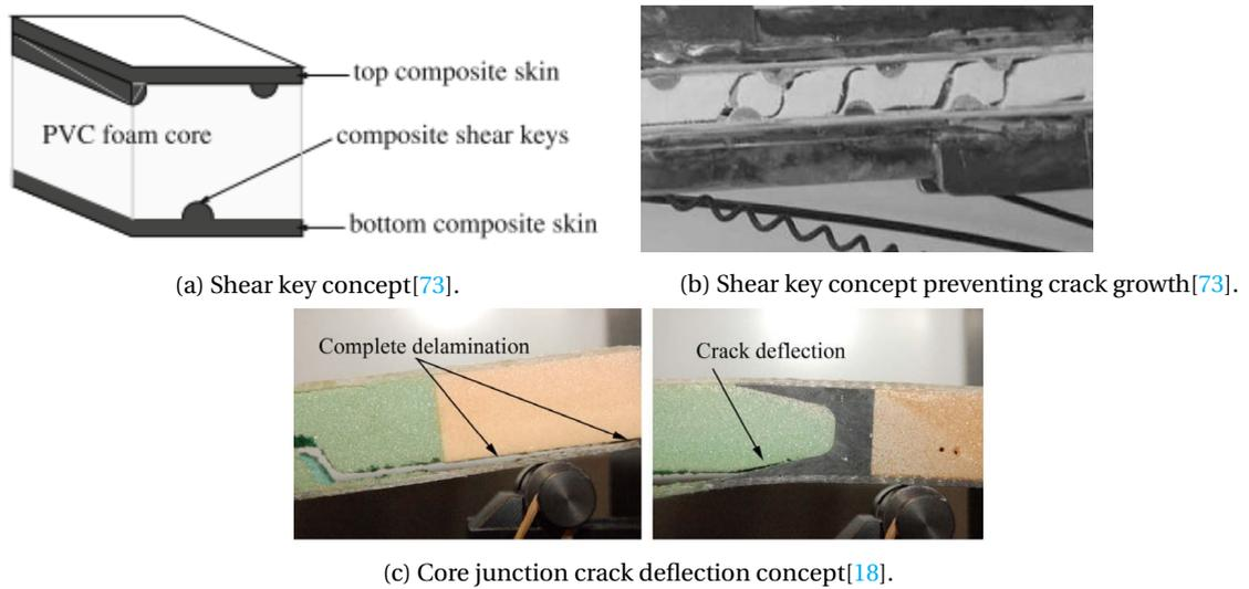
Figure 3.22: Concepts to stop or deflect cracks in sandwich structures
