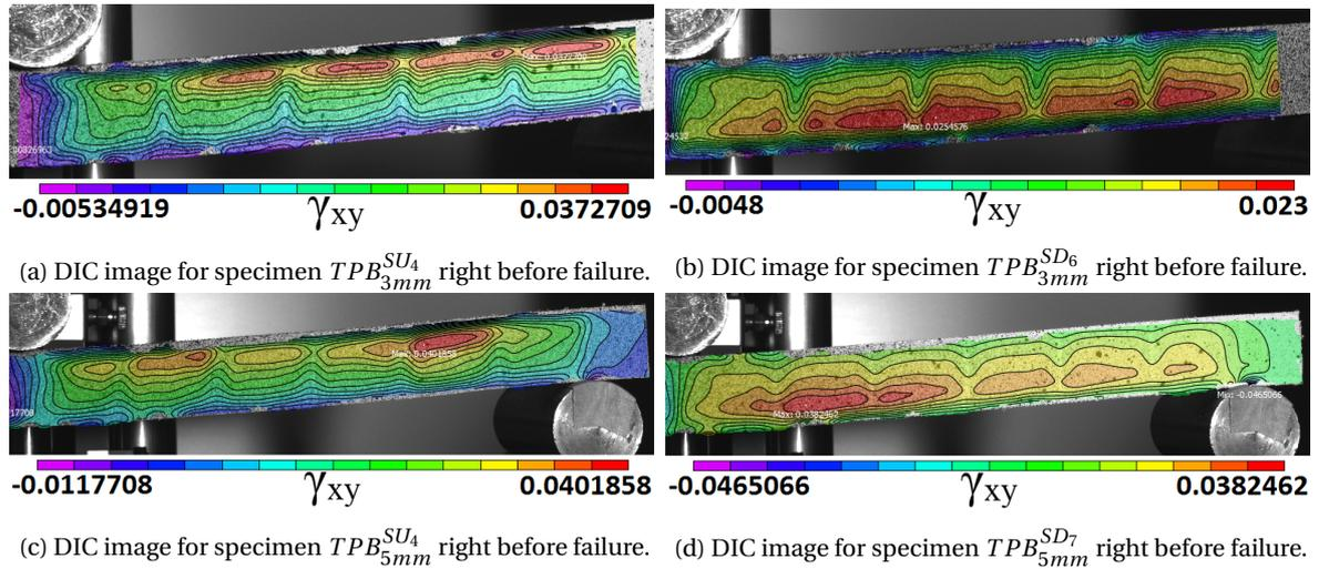
Figure 5.17: DIC Images for the TPB Test of the 3mm and 5mm resin link specimens. All images captured right before failure.
