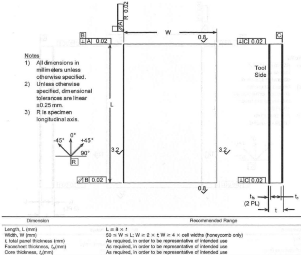
Figure A.16: ASTM C364 coupon dimensions.
