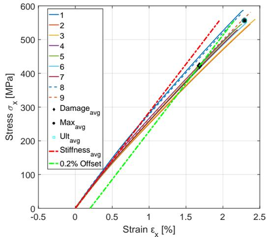
(b) ET test stress vs strain - triax back facing.
