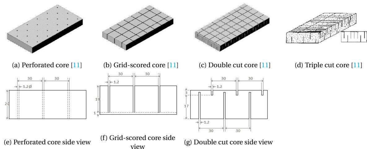
Figure 3.8: Types of contour finishing options for closed-cell sandwich core materials
