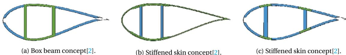
Figure 3.4: General blade design concepts for modern wind turbines.
