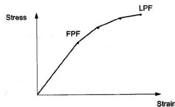
Figure 3.11: First Ply -(FPF) and Last Ply Failure(LPF) - Schematisation of progressive failure analysis[3].
