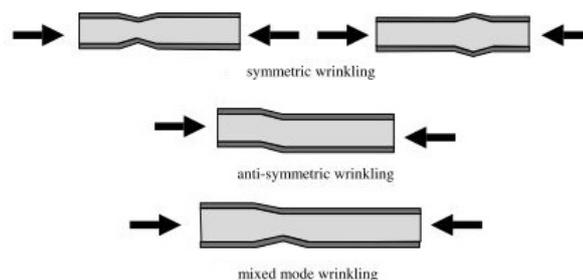
Figure 3.17: Wrinkling types for composite sandwich structures[7].
