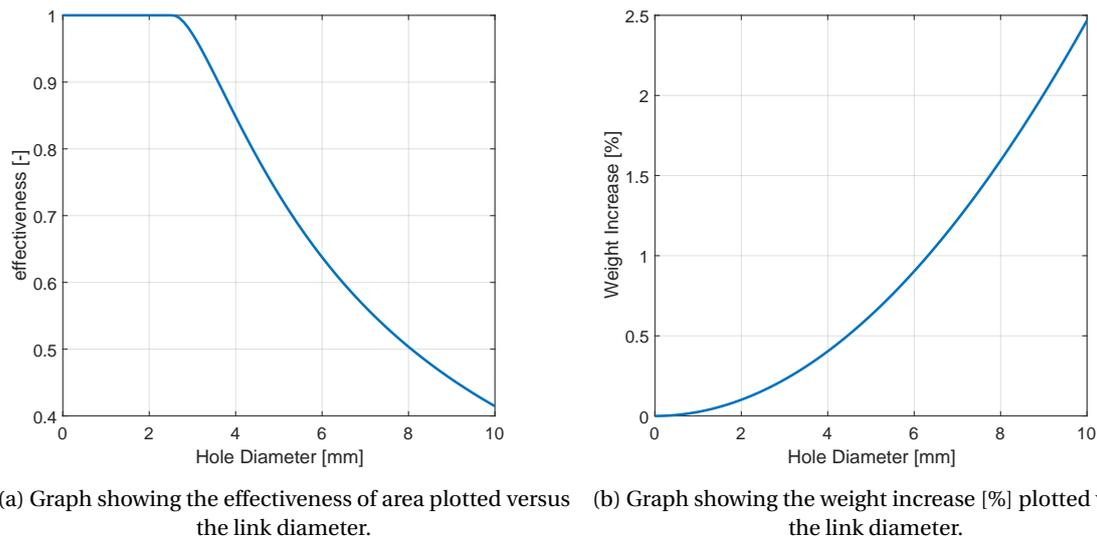
Figure 2.6: Influence of link diameter on effectiveness ratio and weight increase.
