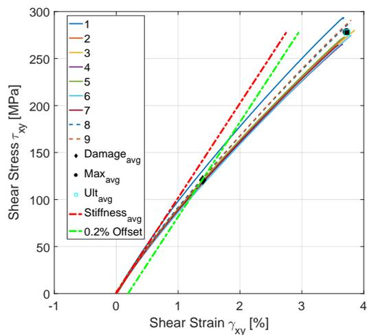
(c) ET test shear stress vs shear strain - triax front facing.
