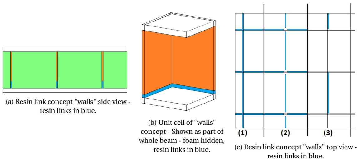
Figure 2.2: Concept "walls" sandwich structure - side and top view - resin links in blue.
