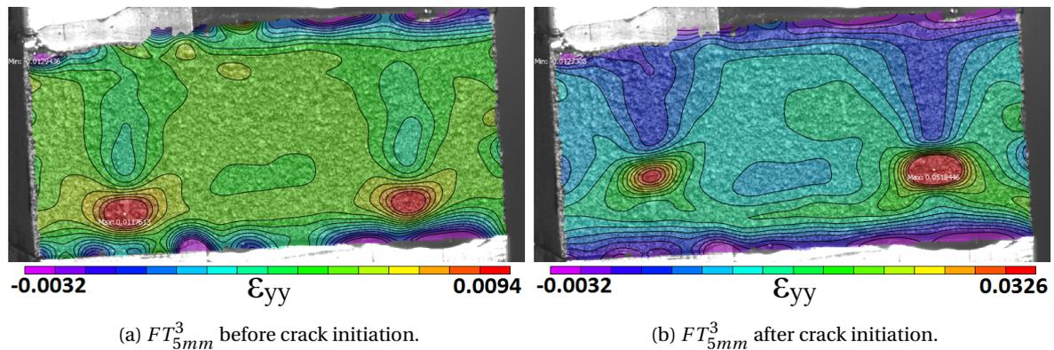
Figure 5.9:  $FT_{5mm}^{10}$  before (left) and after (right) crack initiation.
