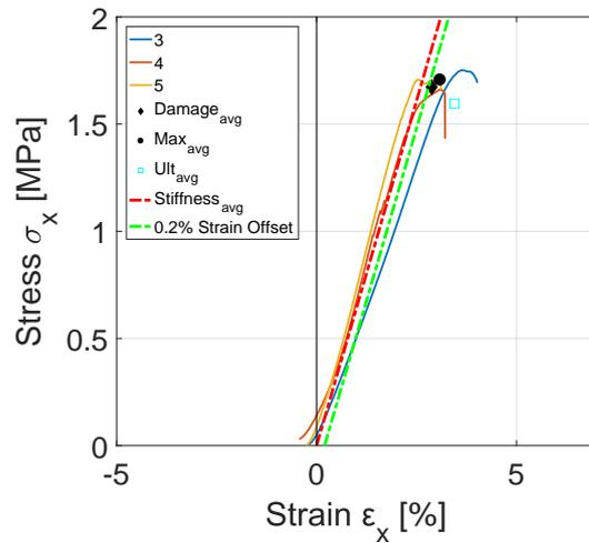
Figure 4.7: Stress-strain curves for FT sandwich specimens.
