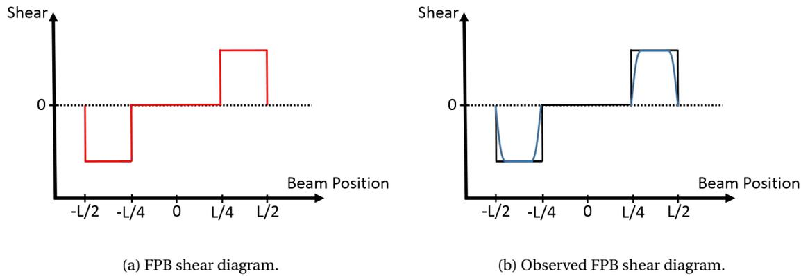
Figure 5.19: 4 point bending shear diagrams.
