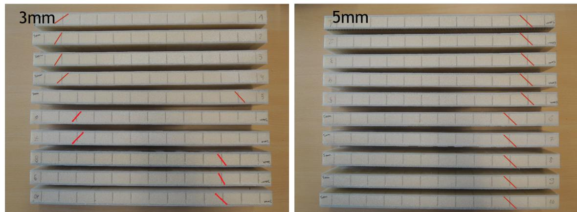
(a) TPB 3mm resin link specimens after failure.
