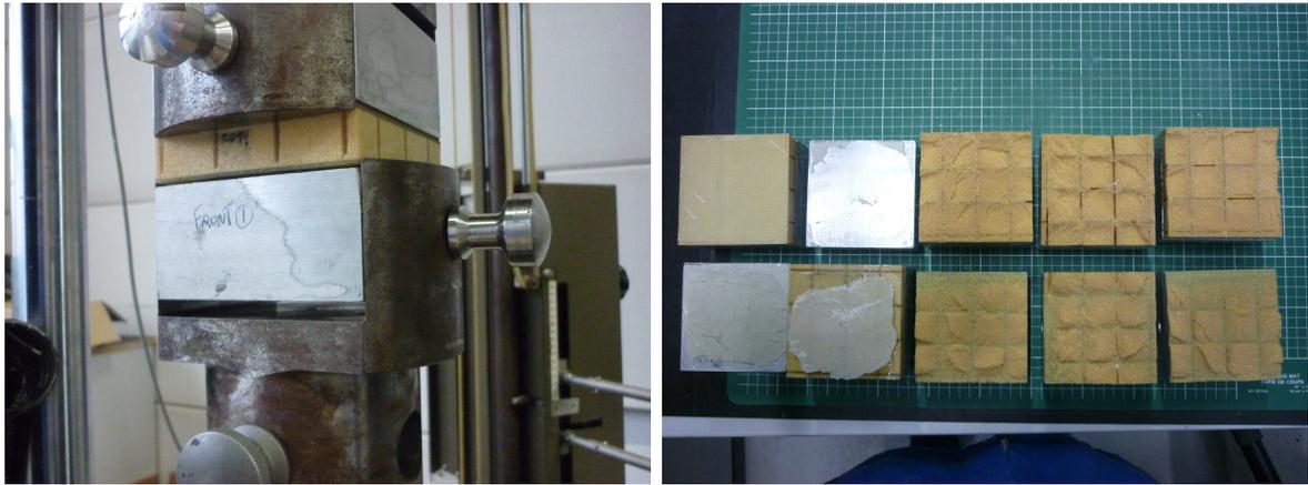
(a) FT specimen during test.
