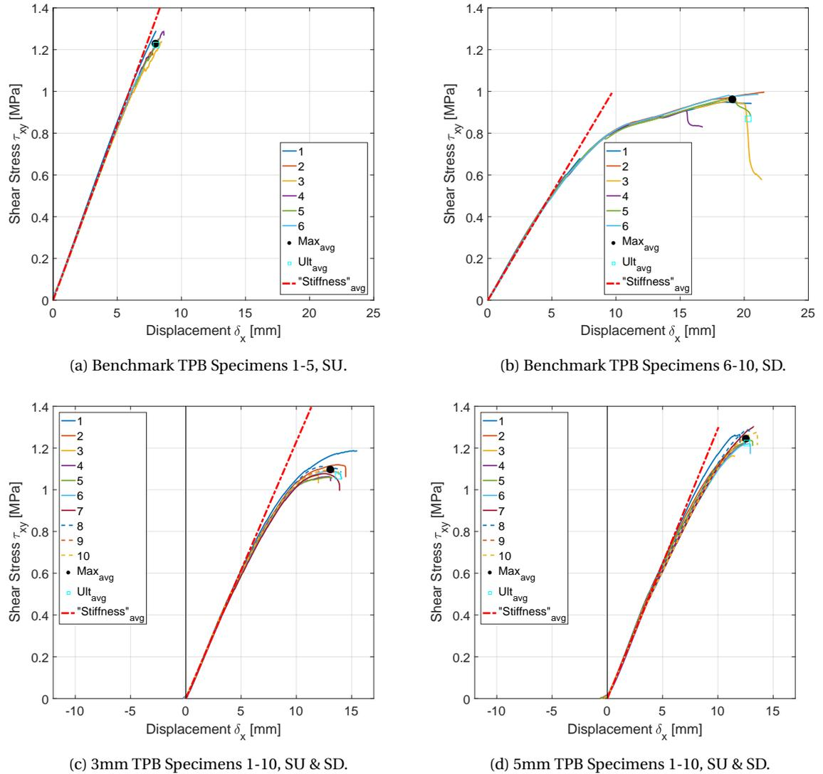
Figure 5.15: Shear stress-displacement graphs for three point bending specimens for benchmark and 3mm and 5mm resin links.
