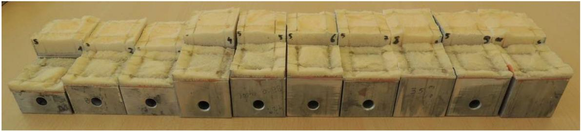
Figure 5.2: Flatwise tension specimens of sandwich structures with 5mm resin links after test.
