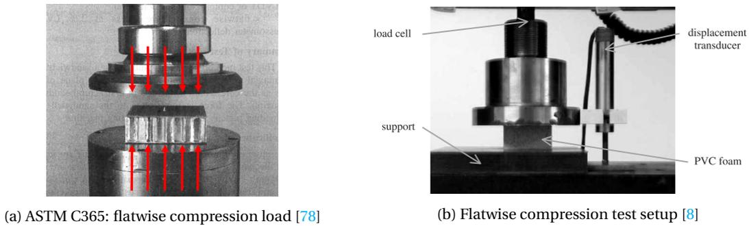
Figure A.10: Flatwise compression test type schematic and test setup picture
