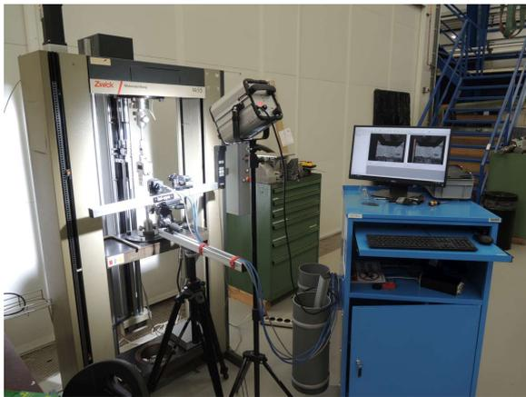
(a) Flatwise tensile test setup.
