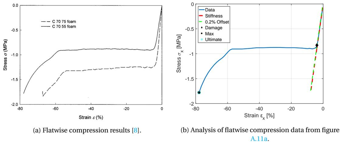
Figure A.11: Flatwise compression stress-strain curves from research by Berthelot et al. [8].
