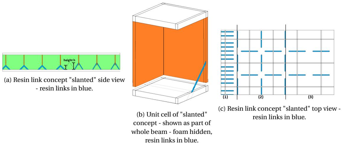
Figure 2.4: Concept "slanted" sandwich structure - side and top view - resin links in blue.
