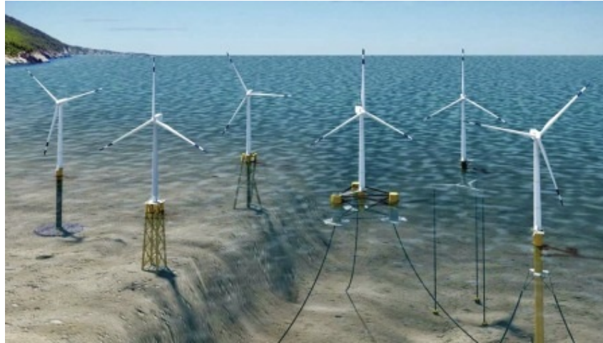
Figure 13: Types of offshore wind turbines, illustration by Josh Bauer, NREL.
