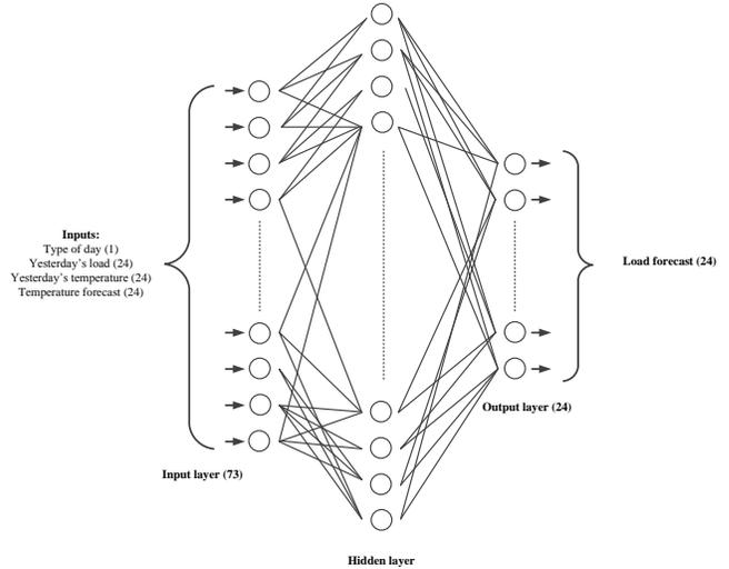
Fig. 2. Neural network architecture for short-term load forecast
