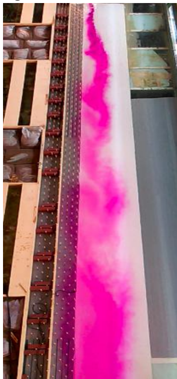
Figure 3.3: The flume experiments are conducted with dyes. The flume is zero-sloped with cylinders on the floodplain. The velocity is measured by ADV along a cross section around 4.5 meters from the beginning of the cylinders.
