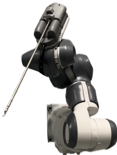
Figure 2. The Smart SATA Driver (SSD) of the AdLap RS. The SSD with the SATA instrument is connected to the YuMi IRB14050 robotic arm (IRB14050, YuMi, ABB, Auburn Hills, MI, USA).
