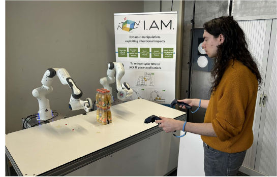
Fig. 2. Depiction of the teleoperation procedure, where a user uses the VIVE handheld controller devices to prescribe a reference for both end effectors.
