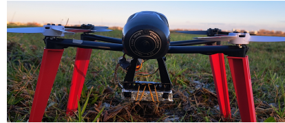
Figure 16: Experimental setup: JeVois stereo camera mounted to the bottom of the drone.
