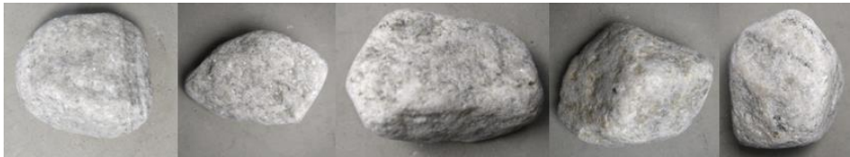
Figure 4-1 Recycle ballast after cleaning
