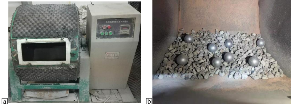
Figure 5-6 Los Angeles Abrasion: (a) Test apparatus, (b) Sample with iron ball inside the chamber
