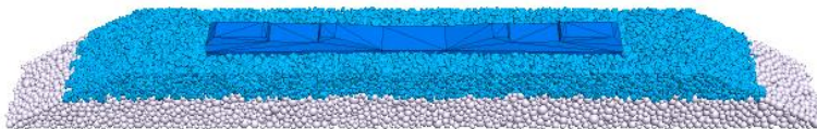
Figure 2-13. Multi-layer model with clumps and balls of a single sleeper section model
