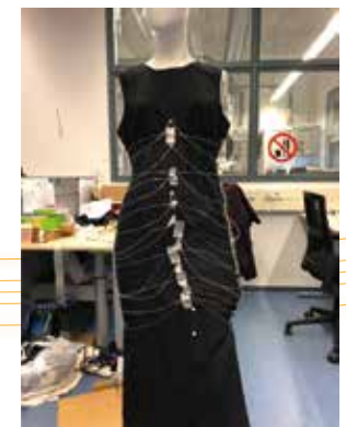
The first rough alignment of the fiber optic wires
