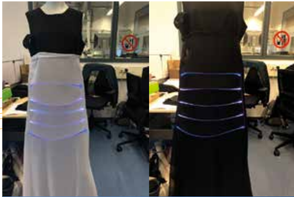
The decision was made to not integrate the fiber optics in the fabric, but rather fixate the optics and the LED's in the dress itself, and cover the lights with fabric that can be moved
