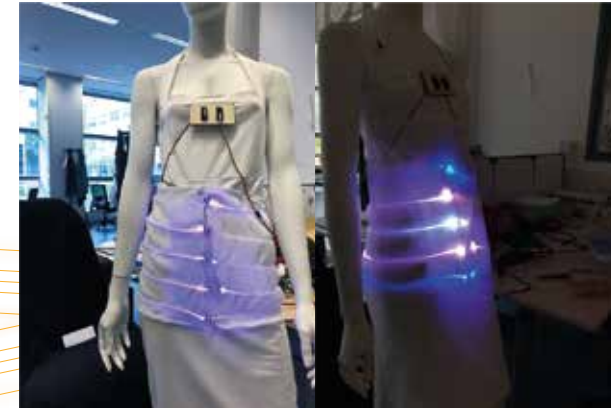
A new set-up, with twice as many lights to have a stronger light diffusion. Also, 2 motors are attached to the middle part for symetrical movements
