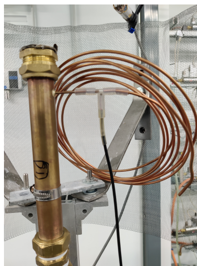
Figure 4-15: Infinity coil connected to the main burner with a microphone installed inline.
