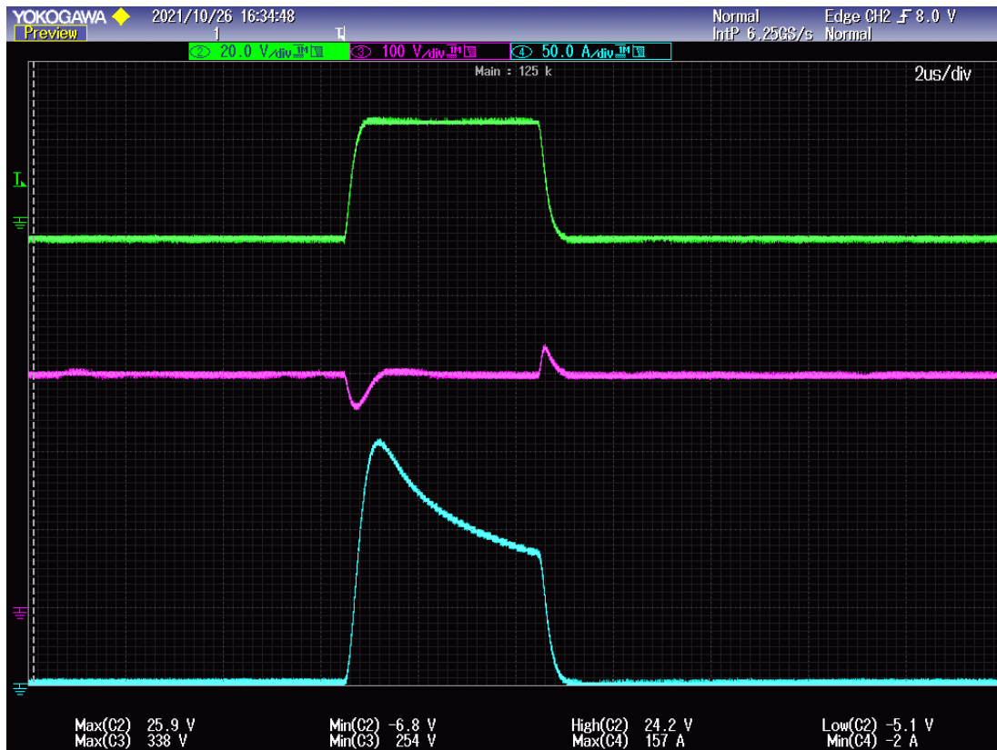
Figure B-2 Oscilloscope image V_{GS} Test (C2M0160120D)
