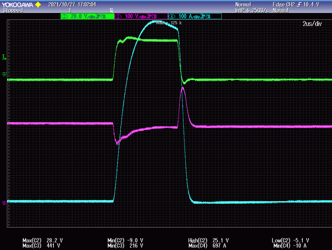
Figure B-10 - TRENCH GATE FS IGBT - IHW40N120R5
