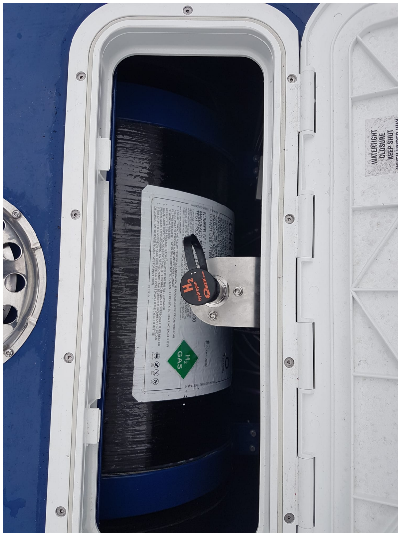
Figure 4.2: Hydrogen storage tank with fuel cap.
