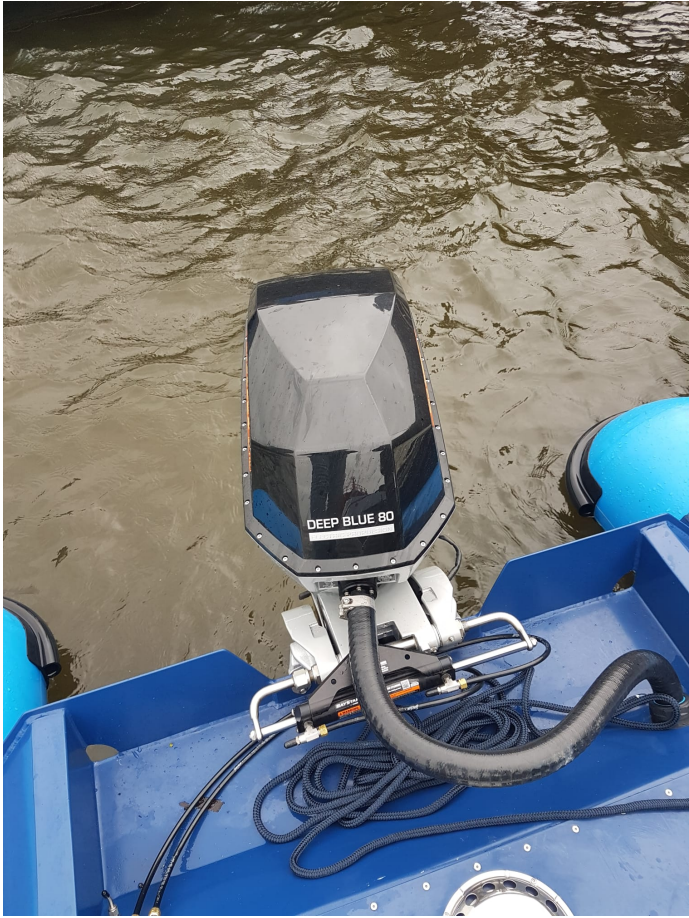
Figure 4.5: Outboard electric propulsion motor Deep Blue 50 Torqeedo.
