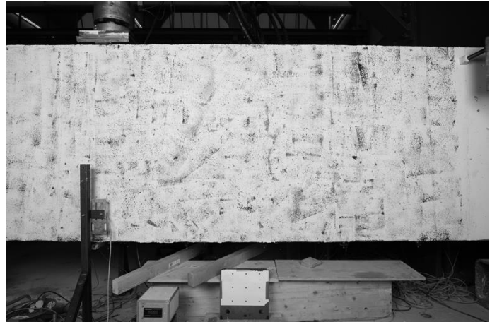
Figure 4. Photo of DIC sprinkle pattern on the other side of the beam.
