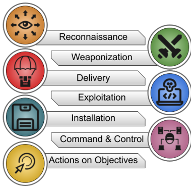
Figure 1.1: The Cyber Kill Chain as introduced by Lockheed Martin [7]. Adversaries have to traverse all stages for a successful attack.
