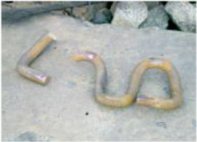
Broken tension clamp Basirat et.al, 2017
