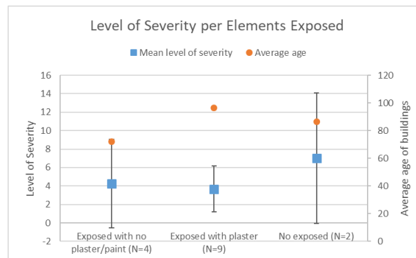
Figure 11. Level of severity per characteristics of exposed RC elements
